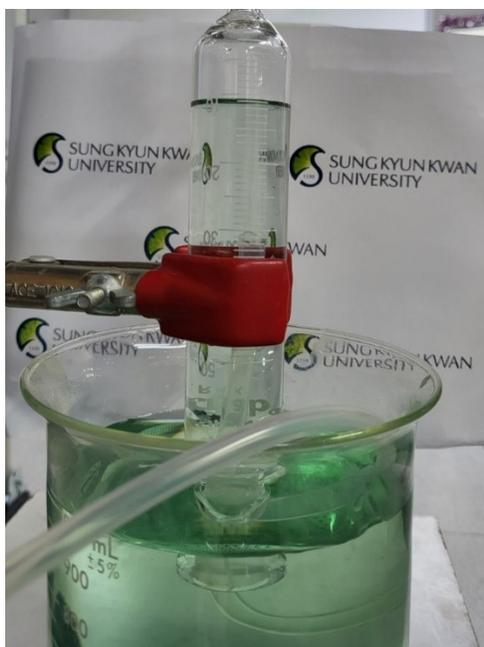
**Figure S6.** Photograph of oxygen gas collection. Oxygen gas is generated during chronopotentiometry at  $20 \text{ mA cm}^{-2}$ .
