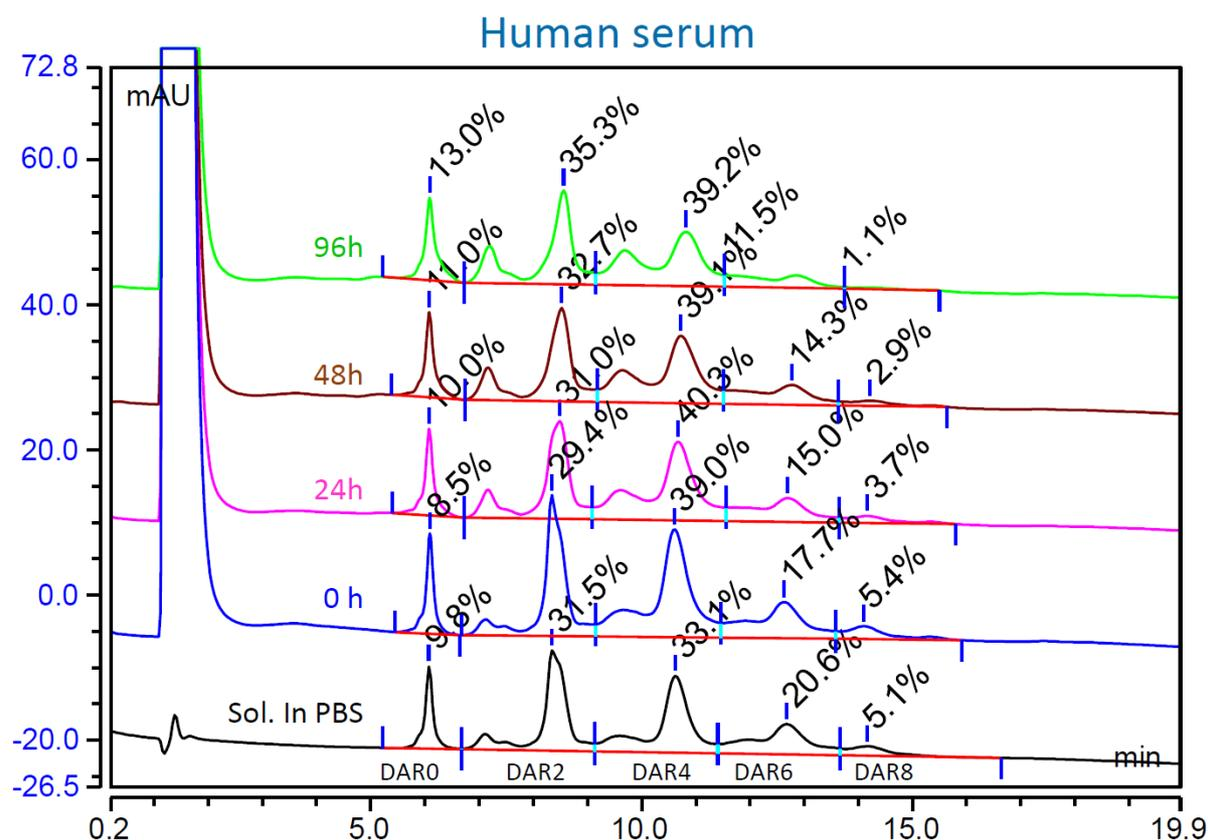
**Figure S8:** Hydrophobic interaction chromatograms at 280 nm of ADC1 incubated at 37 °C in IgG-depleted human serum for 0 h, 24 h, 48 h & 96 h.
