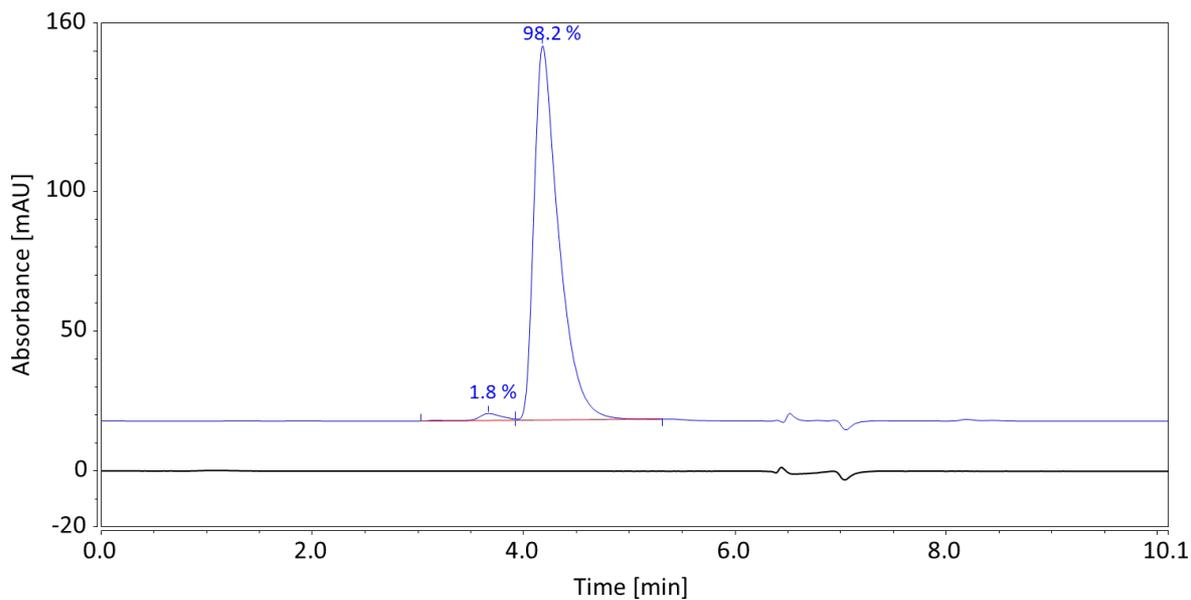
**Figure S5:** Size exclusion chromatogram at 248 nm of ADC1 (blue trace) and PBS blank (black trace)
