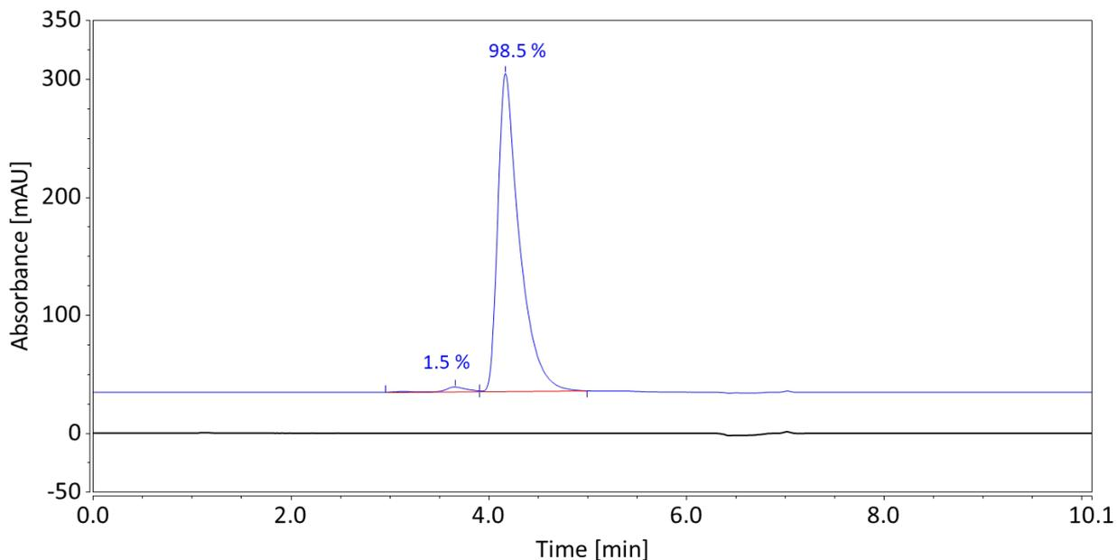
**Figure S2:** Size exclusion chromatogram at 280 nm of ADC1 (blue trace) and PBS blank (black trace)
