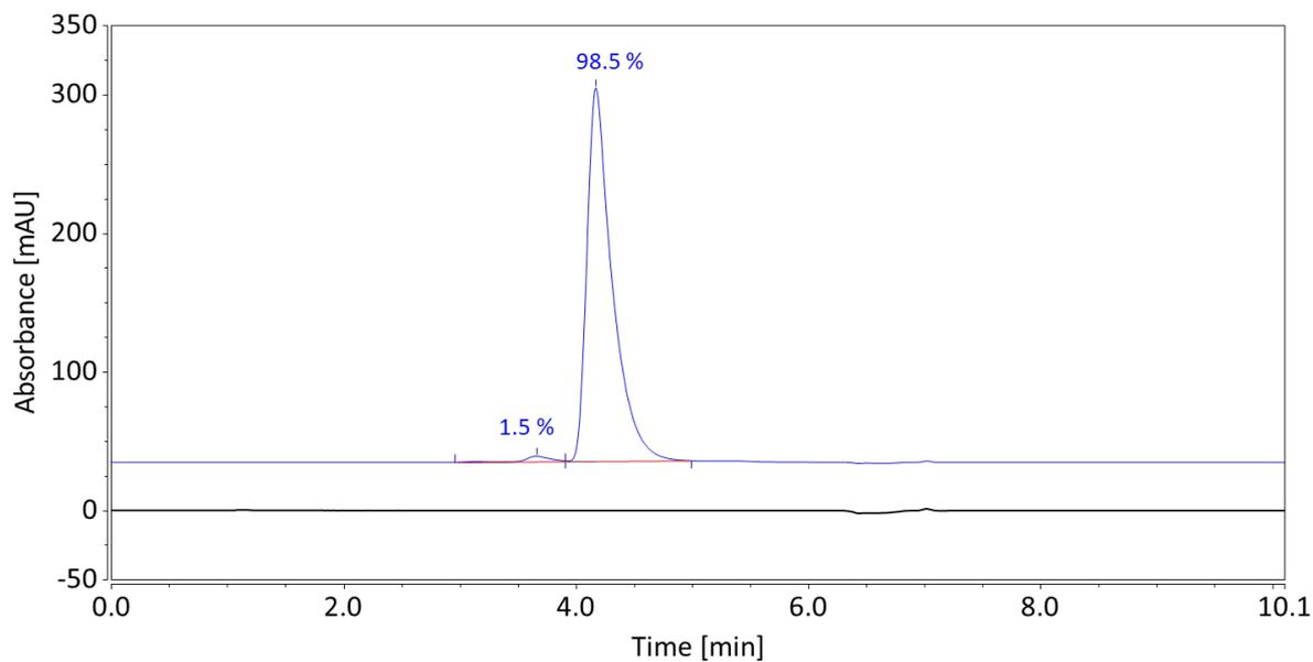
**Figure S4:** Size exclusion chromatogram at 280 nm of ADC1 (blue trace) and PBS blank (black trace)
