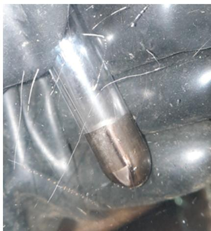
**Fig. S53.** Photograph of the Ge film deposited on the inner wall of the quartz reactor from the photolysis of poly(3,4-dihexylgermacyclopentene-*r*-3,4-diisopropylgermacyclopentene) (**14**) in THF.
