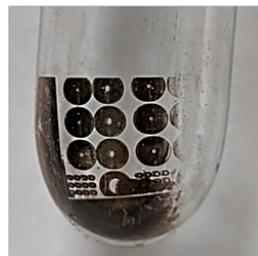
**Fig. S58.** (a) Photograph of the photolysis reactor filled with a solution of poly(3,4-dihexylgerma-cyclopentene) (**13**) in THF pre-photolysis; (b) photograph of the photolysis reactor after photolysis and removal of the photopatterning mask. Deposited germanium shows a pattern on the inner wall of the reactor.
