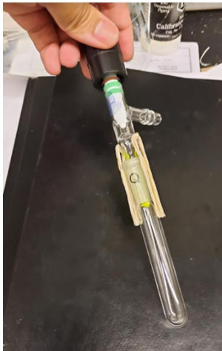
**Fig. S44.** Photograph of the quartz reactor employed for the photolysis of the polymers **11**, **13** and **14** under  $N_2$ .
