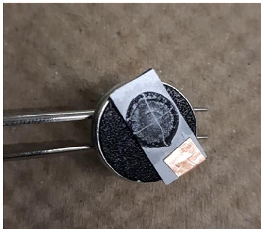
**Fig. S54.** Photograph of the Ge precipitate on a Si wafer for SEM/EDX analysis. The powder was obtained from the photolysis of poly(3,4-dihexylgermacyclopentene-*r*-3,4-diisopropylgermacyclopentene) (**14**) dissolved in THF.
