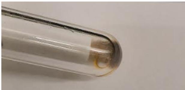
**Fig. S45.** Photograph of the Ge film deposited on the inner wall of the quartz reactor from photolysis of oligo(3,4-dimethylgermacyclopentene) (**11**) in  $THF-d^8$ .
