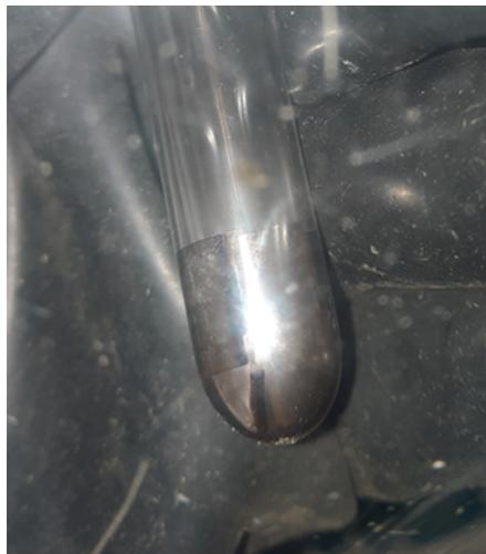
**Fig. S47.** Photograph of the Ge film deposited on the inner wall of the quartz reactor after photolysis of poly(3,4-dihexylgermacyclopentene) (**13**) in THF.
