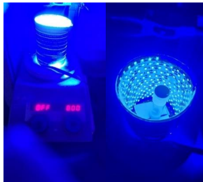
Figure S2. LED light setup
