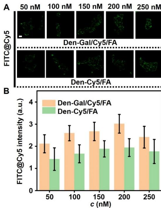
**Fig. S9** (A) Colocalization of FITC fluorescence with Cy5 fluorescence obtained by collecting the FITC fluorescence within Cy5 fluorescence area in Figure S8. Scale bar: 20  $\mu$ m. (B) Statistical FITC@Cy5 intensities from (A). Error bars represent  $\pm$  S.D. (n = 3).
