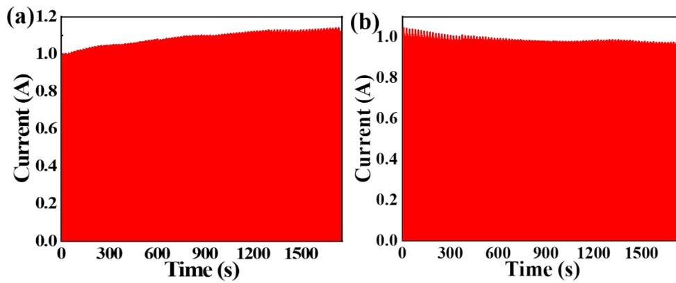
Figure S2 The I-t curve of the CsPbBr<sub>3</sub> PD under 2 mW/cm<sup>2</sup> light: (a) without and with BMIMBr ionic liquid.
