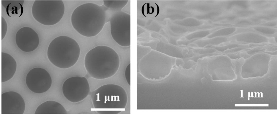
Figure S1 Top (a) and cross-sectional (b) SEM image of the CsPbBr<sub>3</sub> perovskite nanonet film without BMIMBr ionic liquid.
