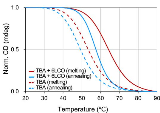
Fig. S5 The CD melting and annealing assay of TBA (2 μM) along at 295 nm (the dotted lines) and TBA with 6LCO (20 μM) at 260 nm (the solid lines) in 50 mM Tris-HCl with 100 mM KCl; Red lines: the melting curve from 20 °C to 90 °C (heating rate: 1 °C/min), Blue lines: the annealing curve from 90 °C to 20 °C (annealing rate: 1 °C/min).
