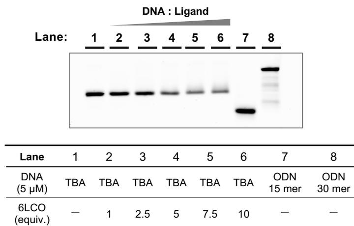
Fig. S2 Native Polyacrylamide Gel assay (20% non-denaturing gel in TBE buffer) of TBA (5  $\mu$ M) with 6LCO (0-50  $\mu$ M; lane: 1-6) and single-stranded DNA, 15 mer and 30 mer, (lane: 7-8) in 50 mM Tris-HCl with 100 mM KCl.
