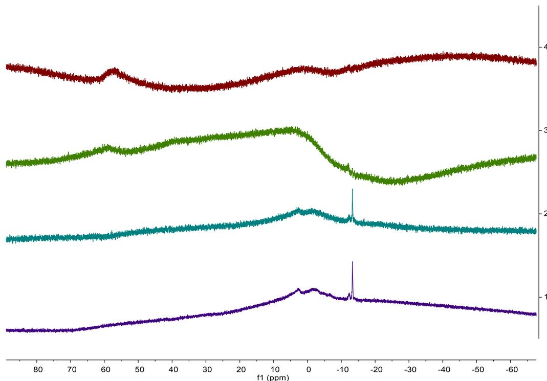
**Fig. S102** The *in-situ*  $^{11}\text{B}$  NMR (128 MHz, 299K,  $\text{C}_6\text{D}_6$ ) spectra of reaction of **1a** with  $\text{PhCH}=\text{CHB}(\text{C}_6\text{F}_5)_2$ . (1) The mixture was heated at 100 °C for 32 h. (2) The mixture was heated at 100 °C for 10 h. (3) The mixture was heated at 80 °C for 10 h. (4) The mixture was heated at 60 °C for 10 h.
