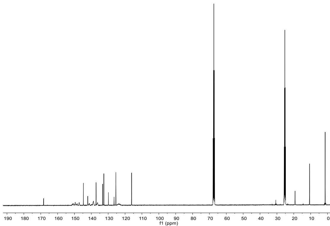
**Fig. S78**  $^{13}\text{C}\{^1\text{H}\}$  NMR (101 MHz, 299K, THF- $d_8$ ) spectrum of compound **4f**.
