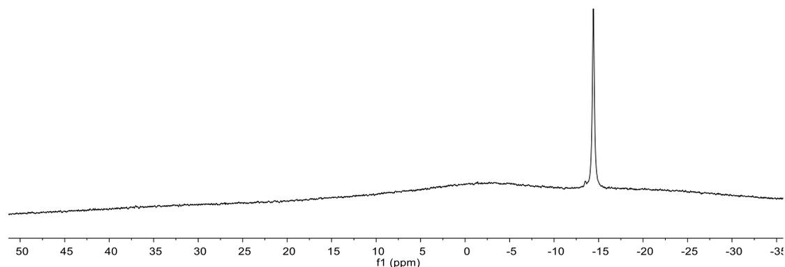
**Fig. S14**  $^{11}\text{B}$  NMR (128 MHz, 299K, THF- $d_8$ ) spectrum of compound **2d**.
