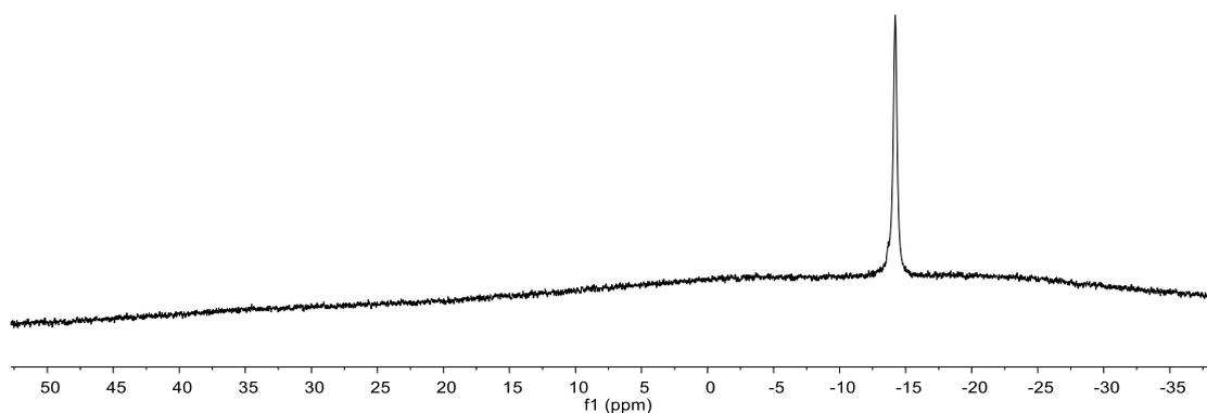
**Fig. S35**  $^{11}\text{B}$  NMR (128 MHz, 299K,  $\text{CD}_2\text{Cl}_2$ ) spectrum of compound **3b**.
