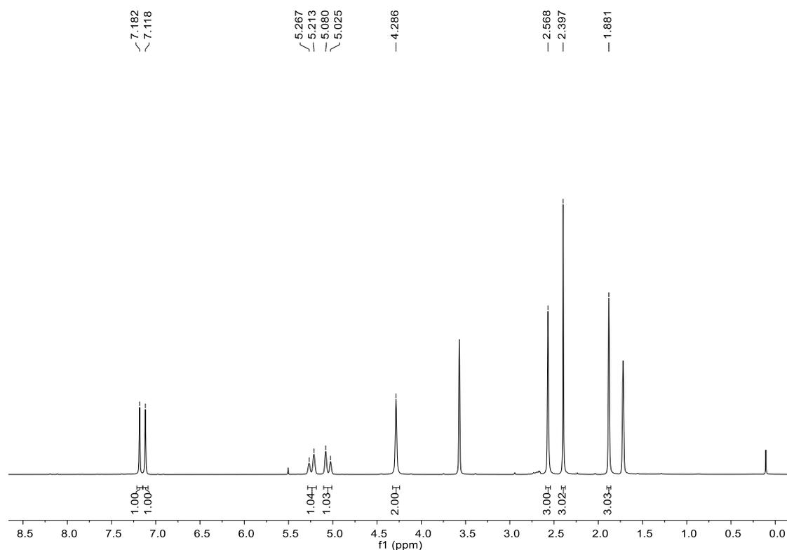
**Fig. S9** <sup>1</sup>H NMR (400 MHz, 299K, THF-d<sub>8</sub>) spectrum of compound **2c**.
