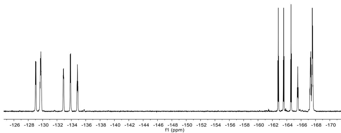
**Fig. S34**  $^{19}\text{F}\{^1\text{H}\}$  NMR (377 MHz, 299K,  $\text{CD}_2\text{Cl}_2$ ) spectrum of compound **3b**.
