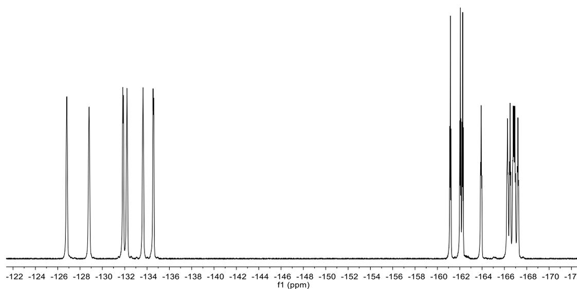
**Fig. S63**  $^{19}\text{F}\{^1\text{H}\}$  NMR (377 MHz, 299K, THF- $d_8$ ) spectrum of compound **4b**.
