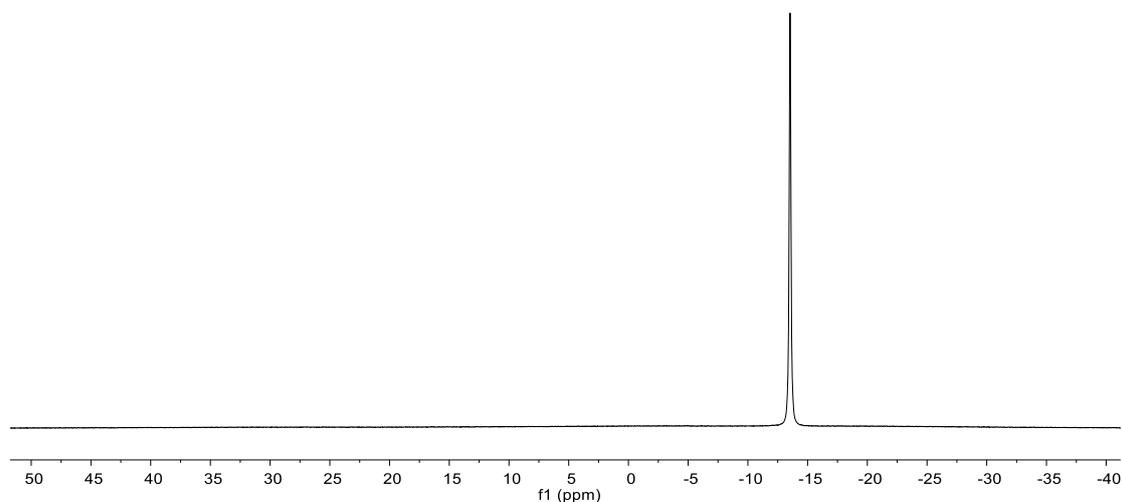
**Fig. S80**  $^{11}\text{B}$  NMR (128 MHz, 299K, THF- $d_8$ ) spectrum of compound **4f**.
