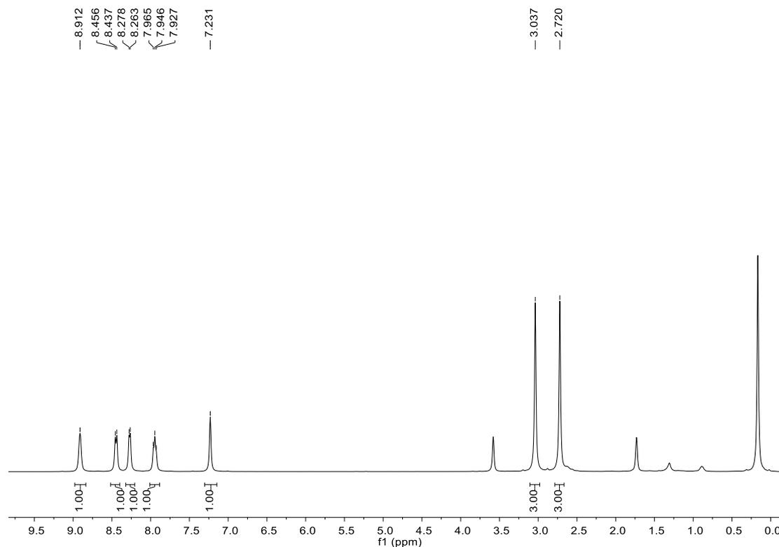
**Fig. S56**  $^1\text{H}$  NMR (400 MHz, 299K, THF- $d_8$ ) spectrum of compound **4a**.
