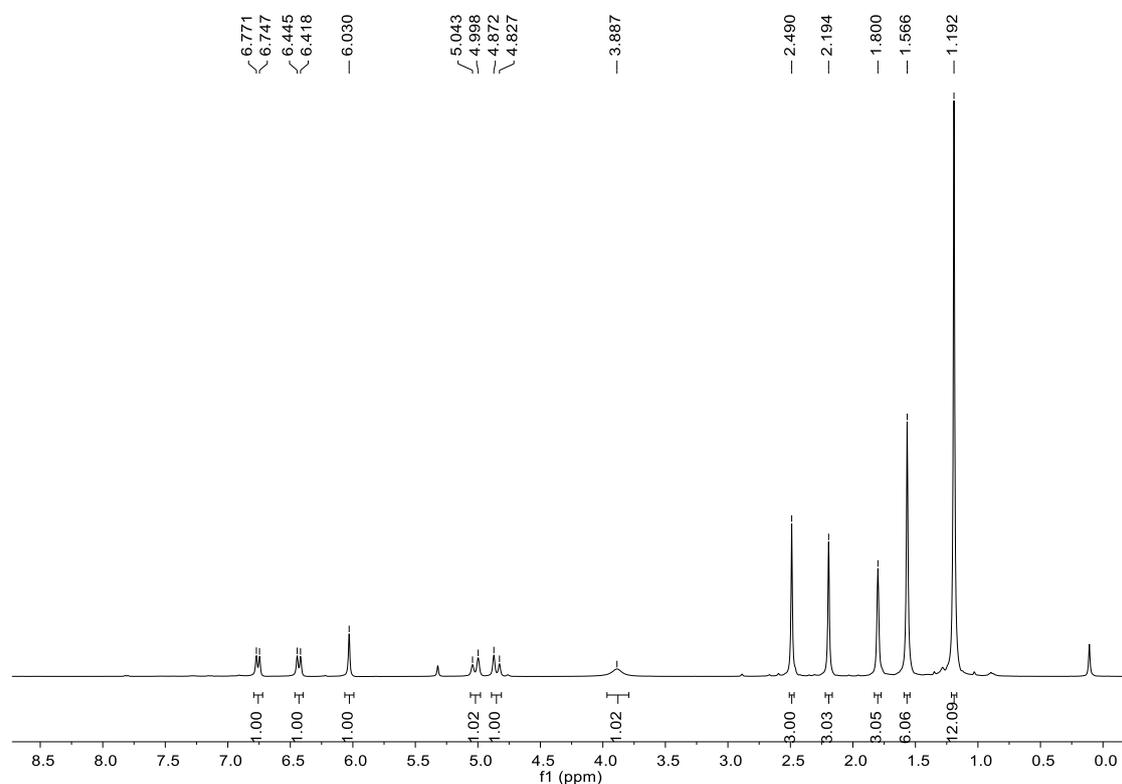
**Fig. S44**  $^1\text{H}$  NMR (400 MHz, 299K,  $\text{CD}_2\text{Cl}_2$ ) spectrum of compound **3e**.
