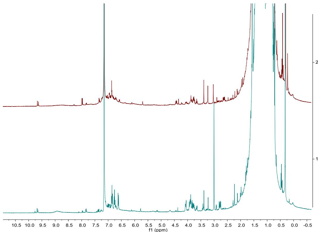
**Fig. S103** The *in-situ*  $^1\text{H}$  NMR (400 MHz, 299K,  $\text{C}_6\text{D}_6$ ) spectra of reaction of **1a** with  $\text{BBr}_3$ . (1) The reaction of **1a** with  $\text{BBr}_3$  in a 1:2 molar ratio. (2) The reaction of **1a** with  $\text{BBr}_3$  in a 1:1 molar ratio.
