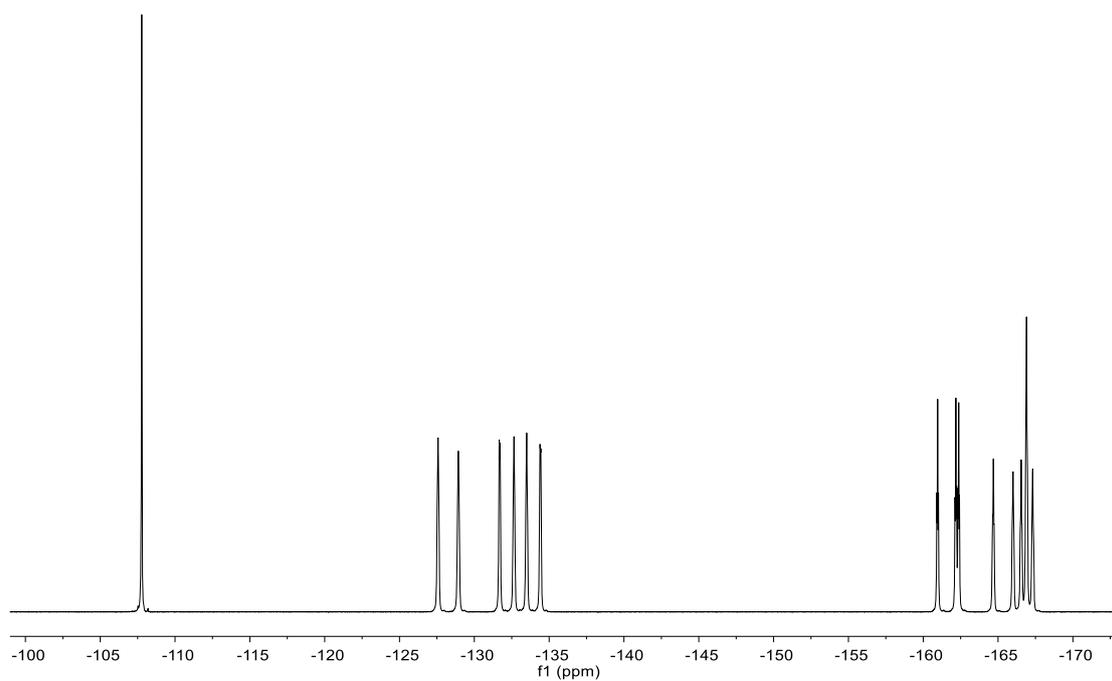
**Fig. S75**  $^{19}\text{F}\{^1\text{H}\}$  NMR (377 MHz, 299K, THF- $d_8$ ) spectrum of compound **4e**.
