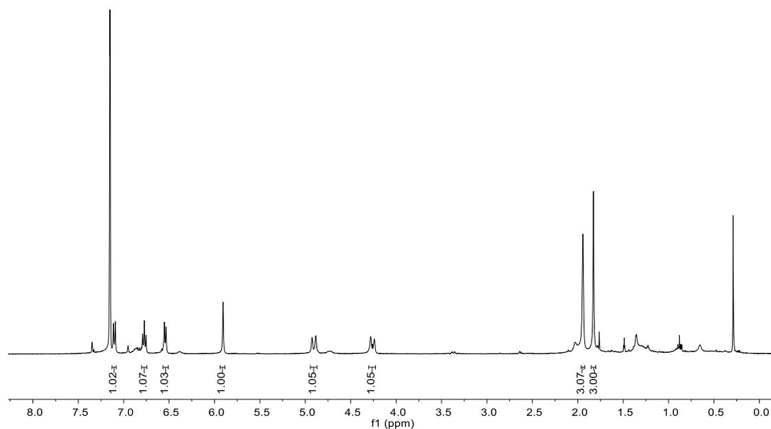
**Fig. S94** The *in-situ*  $^1\text{H}$  NMR (400 MHz, 299K,  $\text{C}_6\text{D}_6$ ) spectrum of reaction of **2a** and  $\text{Cs}_2\text{CO}_3$ .
