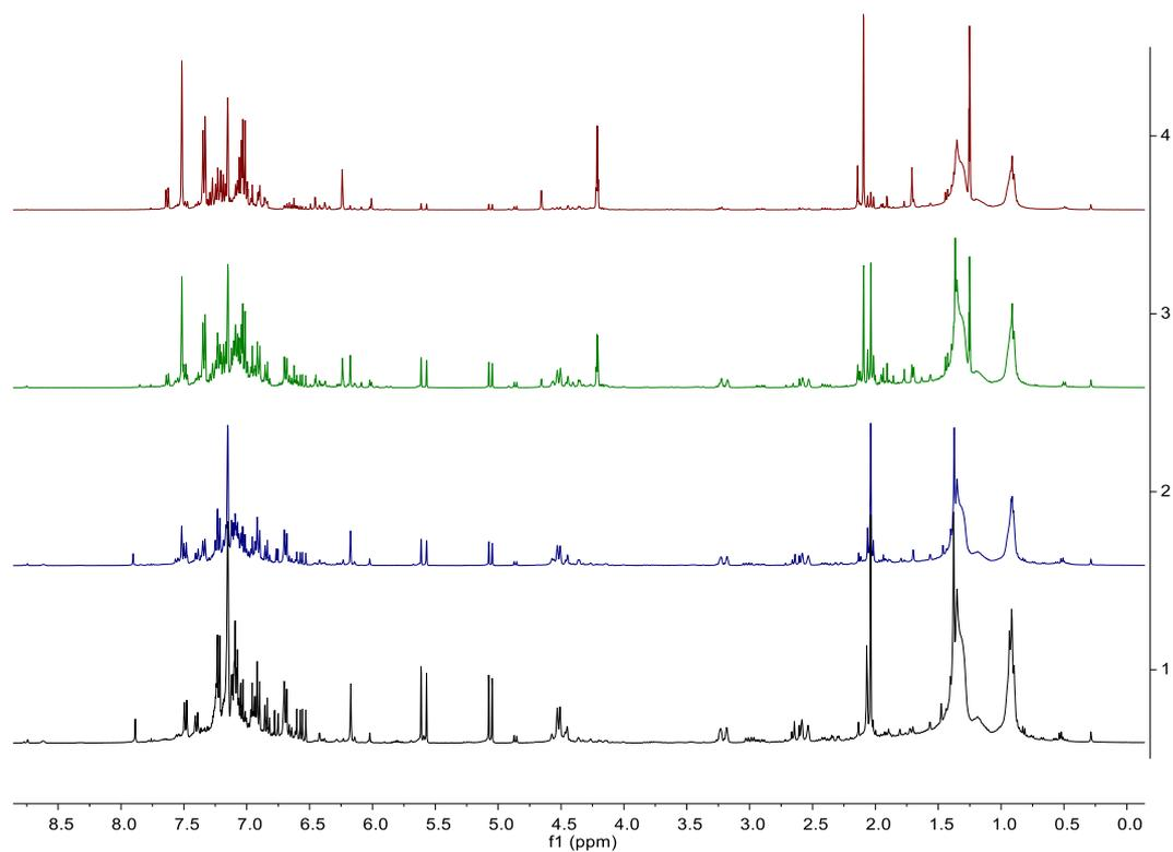
**Fig. S100** The *in-situ* <sup>1</sup>H NMR (400 MHz, 299K, C<sub>6</sub>D<sub>6</sub>) spectra of reaction of **1a** with PhCH=CHB(C<sub>6</sub>F<sub>5</sub>)<sub>2</sub>. (1) The mixture was heated at 100 °C for 32 h. (2) The mixture was heated at 100 °C for 10 h. (3) The mixture was heated at 80 °C for 10 h. (4) The mixture was heated at 60 °C for 10 h.
