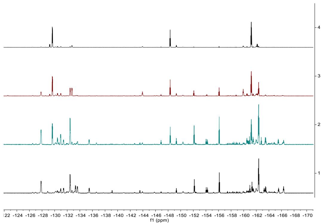
**Fig. S101** The *in-situ*  $^{19}\text{F}\{^1\text{H}\}$  NMR (377 MHz, 299K,  $\text{C}_6\text{D}_6$ ) spectra of reaction of **1a** with  $\text{PhCH}=\text{CHB}(\text{C}_6\text{F}_5)_2$ . (1) The mixture was heated at 100 °C for 32 h. (2) The mixture was heated at 100 °C for 10 h. (3) The mixture was heated at 80 °C for 10 h. (4) The mixture was heated at 60 °C for 10 h.
