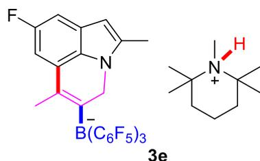
According to the General Procedure II (for **3**) from **2e** (142.7 mg, 0.2 mmol) and PMP (31.1 mg, 0.2 mmol). The product **3e** was isolated as a yellow solid (147.7 mg, 85% yield).
