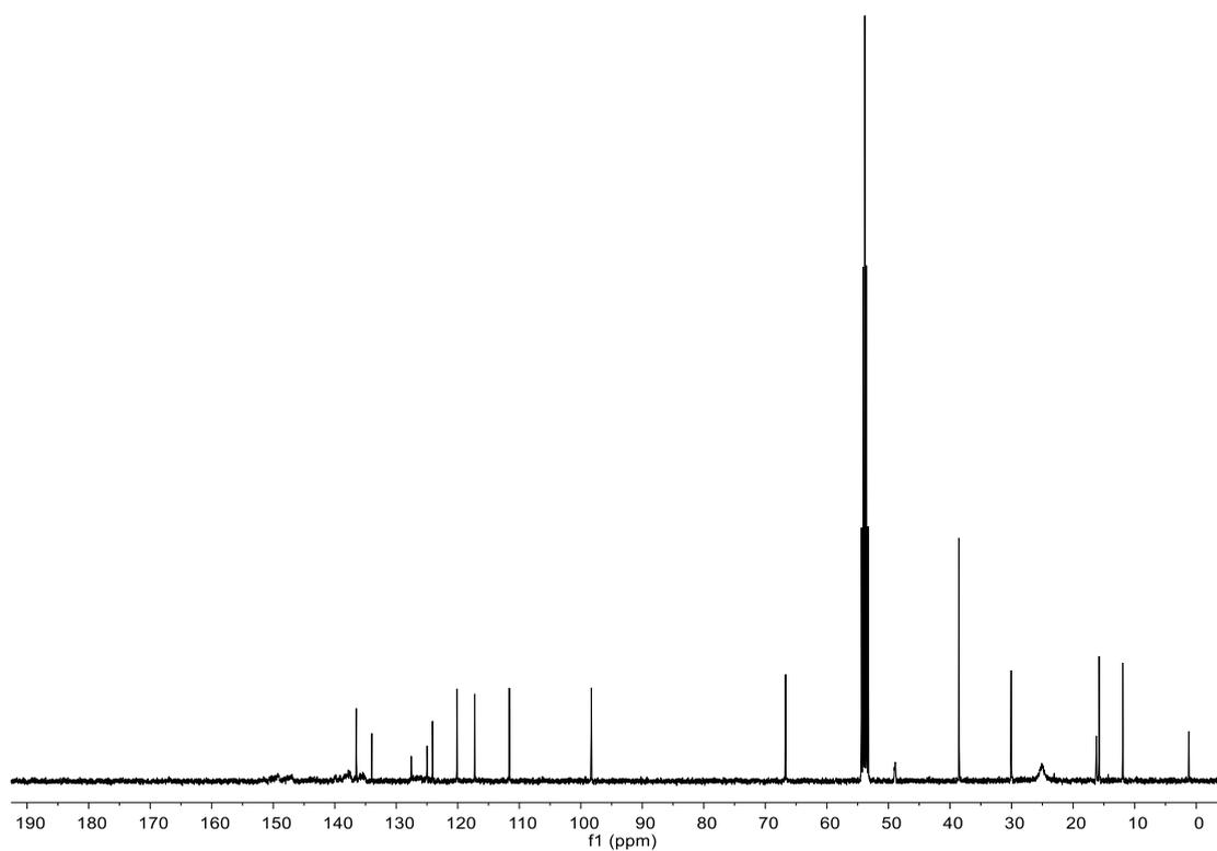
**Fig. S28**  $^{13}\text{C}\{^1\text{H}\}$  NMR (101 MHz, 299K,  $\text{CD}_2\text{Cl}_2$ ) spectrum of compound **3a**.
