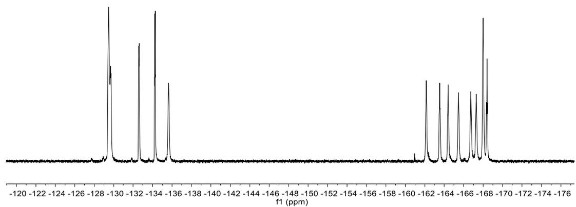
**Fig. S19**  $^{19}F\{^1H\}$  NMR (377 MHz, 299K, THF- $d_8$ ) spectrum of compound **2f**.
