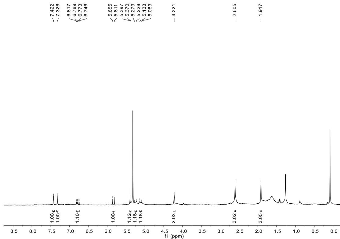
**Fig. S24**  $^1\text{H}$  NMR (400 MHz, 299K,  $\text{CD}_2\text{Cl}_2$ ) spectrum of compound **2h**.
