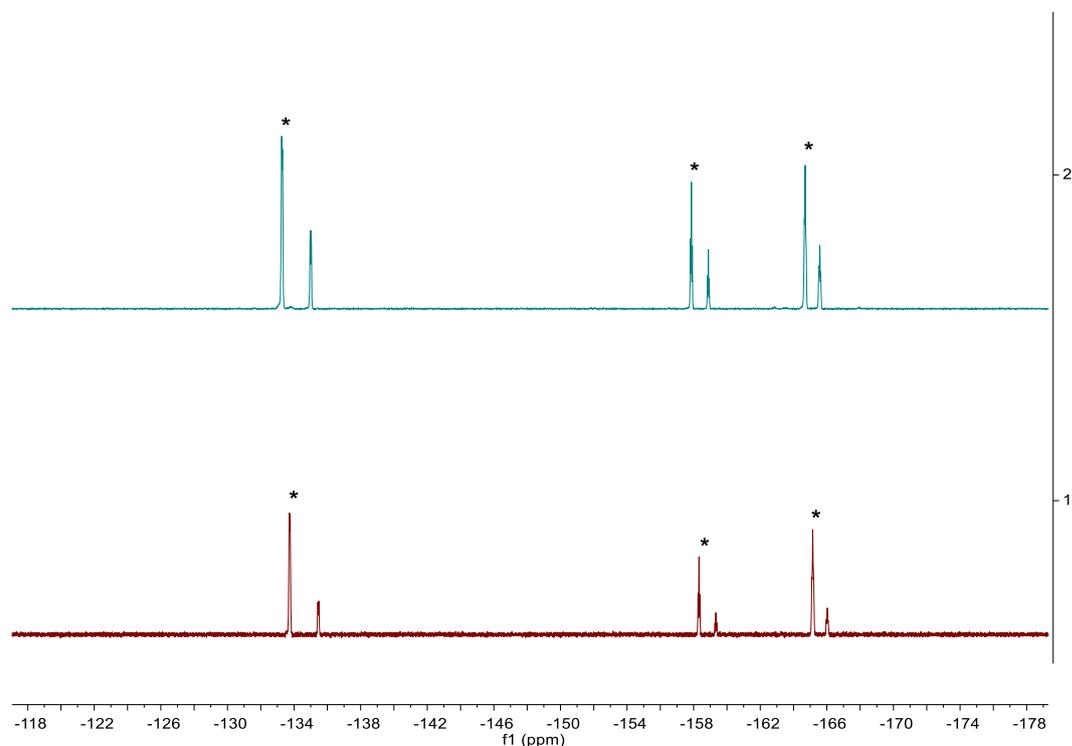
**Fig. S105** The *in-situ*  $^{19}\text{F}\{^1\text{H}\}$  NMR (377 MHz, 299K, THF) spectra of reaction of **1f** with 20 mol%  $\text{B}(\text{C}_6\text{F}_5)_3$ . (1) The mixture was heated at 100 °C for 11 h. (2) The mixture was heated at 80 °C for 11 h. [\*  $(\text{C}_6\text{F}_5)_3\text{B}\cdot\text{THF}$  Lewis acid-base adduct]
