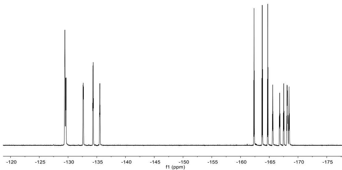
**Fig. S10**  $^{19}\text{F}\{^1\text{H}\}$  NMR (377 MHz, 299K, THF- $d_8$ ) spectrum of compound **2c**.
