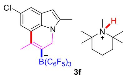
According to the General Procedure II (for **3**) from **2f** (146.0 mg, 0.2 mmol) and PMP (31.1 mg, 0.2 mmol). The product **3f** was isolated as a white solid (146.9 mg, 83% yield).
