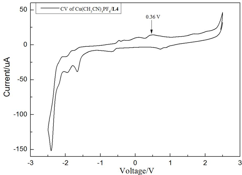
**Figure S6** Cyclic voltammograms of  $\text{Cu}(\text{CH}_3\text{CN})_4\text{PF}_6/\text{L4}$  (generated in situ by stirring a 1:1 mixture of  $\text{Cu}(\text{CH}_3\text{CN})_4\text{PF}_6$  and ligand **L4**) in  $\text{CH}_3\text{CN}$ .
