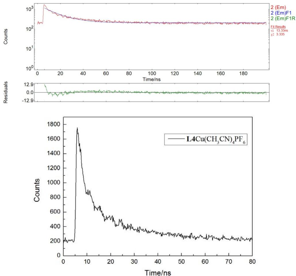
**Figure S5** Lifetime chromatogram of  $\text{Cu}(\text{CH}_3\text{CN})_4\text{PF}_6/\text{L4}$  excited at 405 nm EPL, 0.0002 M solution in  $\text{CH}_3\text{CN}$  (recorded on an Edinburgh Instrument FLS1000).
