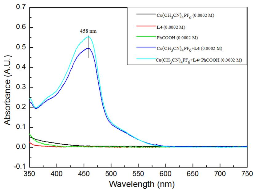
**Figure S1** UV-vis spectrum of the  $\text{Cu}(\text{CH}_3\text{CN})_4\text{PF}_6$  in DCM, **L4** in DCM,  $\text{PhCOOH}$  in DCM,  $\text{Cu}(\text{CH}_3\text{CN})_4\text{PF}_6 + \text{L4}$  in DCM and  $\text{Cu}(\text{CH}_3\text{CN})_4\text{PF}_6 + \text{L4} + \text{PhCOOH}$  in DCM, the peak at 458 nm.
