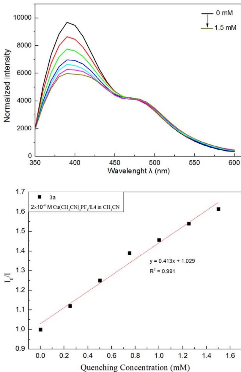
**Figure S4** Stern–volmer quenching studies of  $\text{Cu}(\text{CH}_3\text{CN})_4\text{PF}_6/\text{L4}$  by **3**
