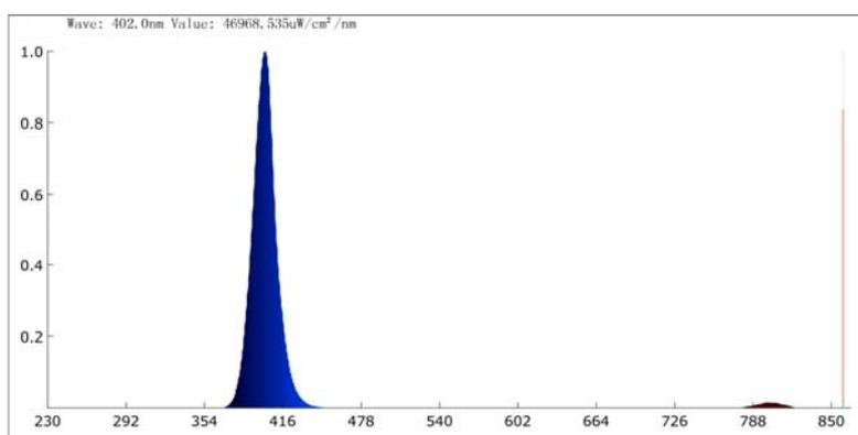
Emission spectra of the 10 W blue LED lamp (maximum emission at  $\lambda = 402$  nm). Wave length: 395 nm-405 nm Quartz glass was used as reaction vessel. Distance between light source and quartz tube was approximately 0.5 cm and no filter was used for the reaction.
