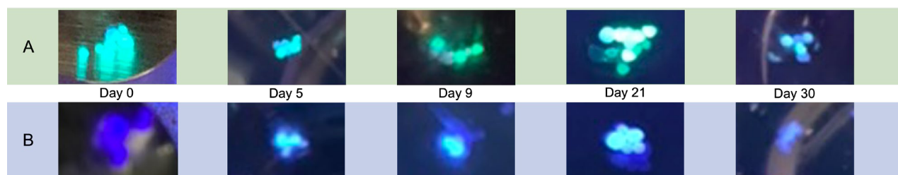
Figure S15. Photographs of (A) 370PC@CsPbBr 3 and (B) 190PC@CsPbBr 1.5 Cl 1.5 microbead hybrids after being submerged in water under a UV lamp (365 nm).
