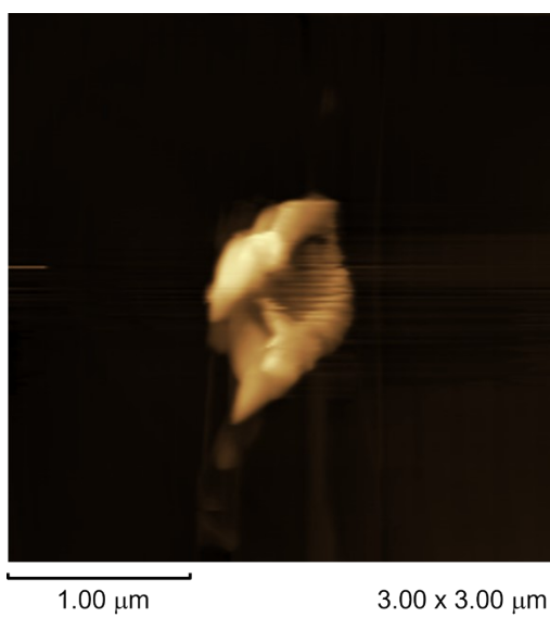
Figure S2. AFM image of sumanene (95.3 \mu\text{M} ) prepared from the MCH solution on an HOPG surface.
