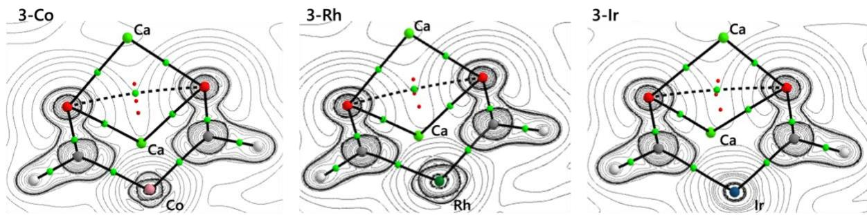
**Figure S27.** QTAIM contour plots of  $\rho$  for **3**. Bond critical points ( $\rho$ ) are shown as green dots, ring critical points as red dots. Carbon, oxygen, and hydrogen atoms are in grey, red, and white respectively. QTAIM charges are tabulated below.
