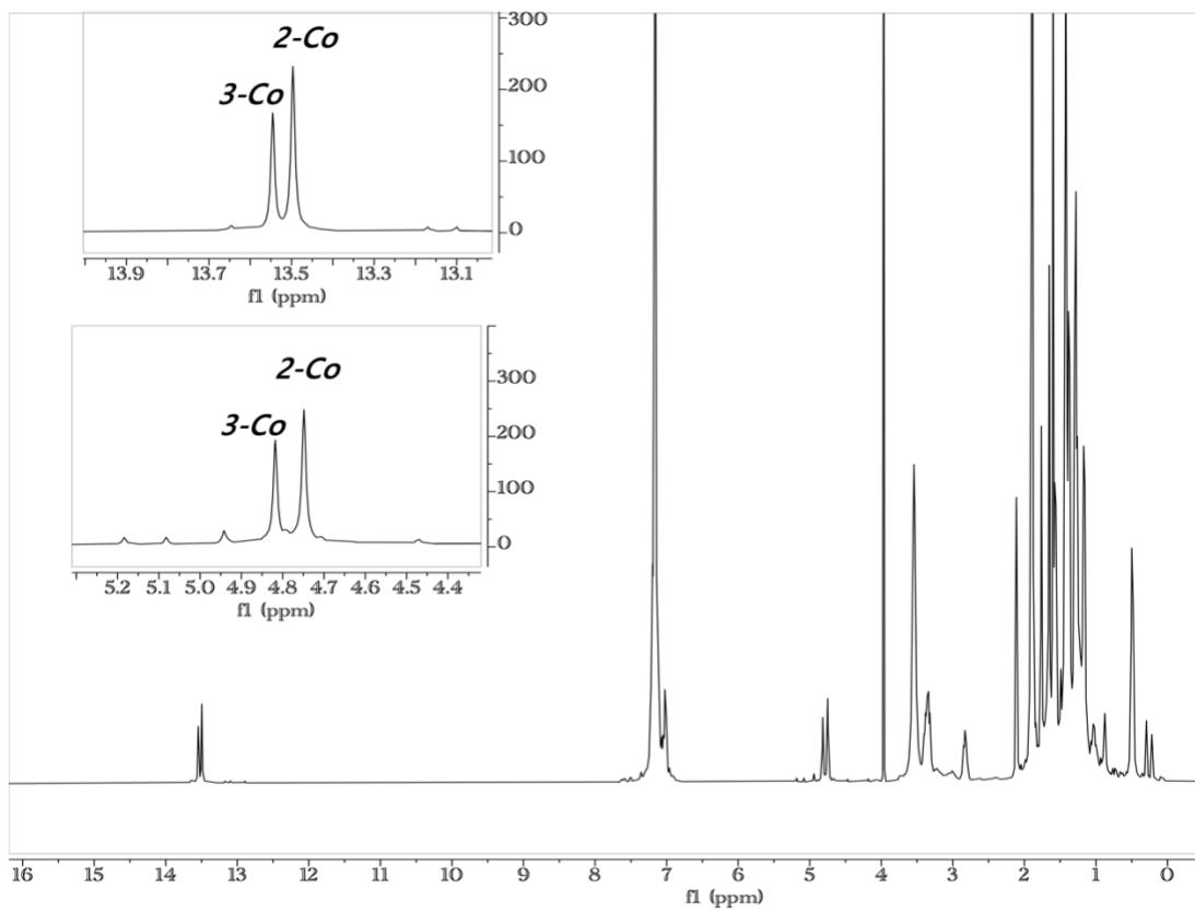
**Figure S1.** <sup>1</sup>H NMR spectra for a **2-Co** and **3-Co** mixture from reaction of **1** and [CoCp\*(CO)<sub>2</sub>] in C<sub>6</sub>D<sub>6</sub> solution.
