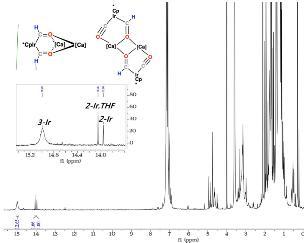
**Figure S5.**  $^1H$  NMR spectra for a **2-Ir.THF** and **3-Ir** mixture from reaction of **1** and  $[IrCp^*(CO)_2]$  in  $C_6D_6$  solution.
