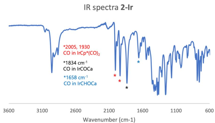
**Figure S13.** Infrared spectra of **2-Ir**.
