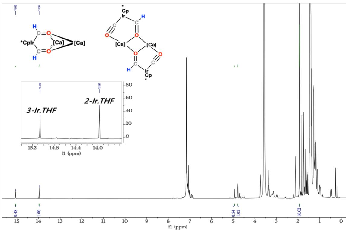
**Figure S6.**  $^1\text{H}$  NMR spectra for a **2**-Ir.thf and **3**-Ir.thf mixture from reaction of **1** and  $[\text{IrCp}^*(\text{CO})_2]$  in  $\text{C}_6\text{D}_6$  solution with THF (0.1 mL) added.
