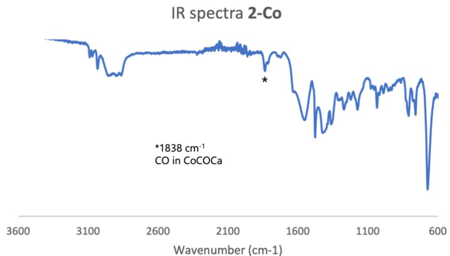
**Figure S11.** Infrared spectra of **2-Co**.
