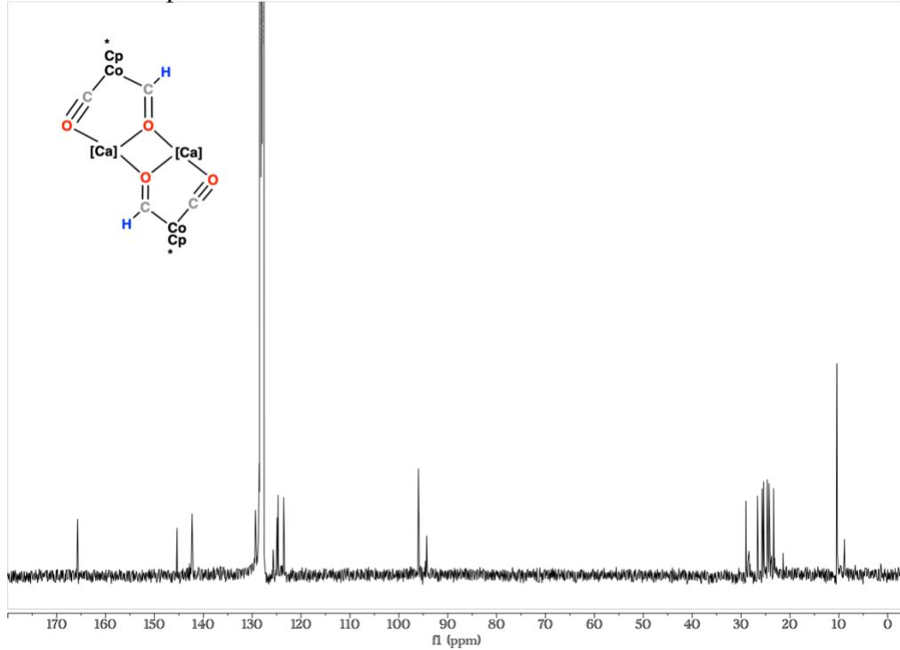
**Figure S15.**  $^{13}\text{C}\{^1\text{H}\}$  NMR spectra of 2-Co.
