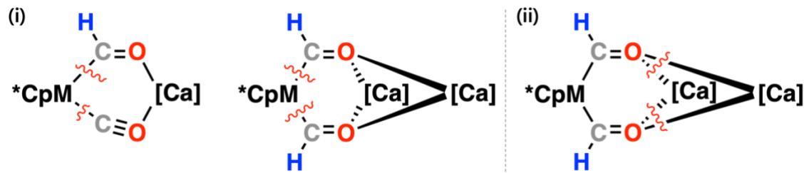
**Figure S28.** Splitting of fragments for ETS-NOCV calculations for complexes **2'** and **3**.
