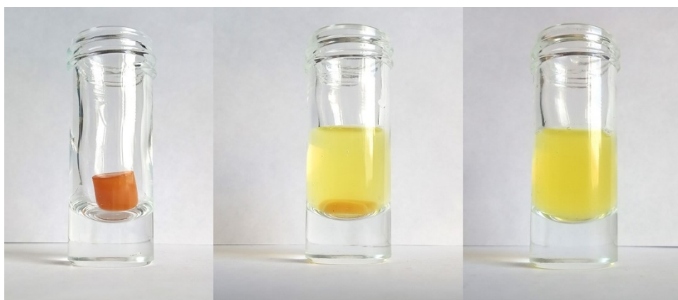
Figure S4. From left to right: Original sample of FeAlg2 hydrogel; residual sample after 10 min in aqueous sodium citrate; completely dissolved sample after 20 min.
