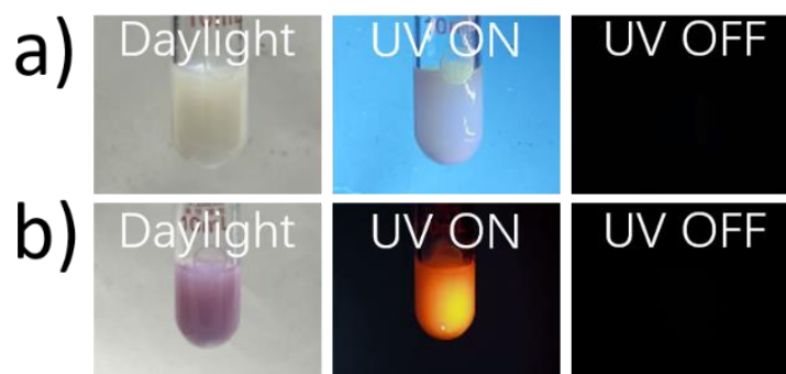
Figure S11. a) Photographs of PMMA and b) SpirocurBF 2 -PMMA emulsions obtained under 365 nm UV and after switching-off the UV lamp at room temperature.
