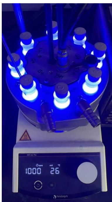
Figure S1. The Reaction Equipment and Light Source ( \lambda_{\text{max}} = 455 \text{ nm} , \Delta\lambda = 25 \text{ nm} )
