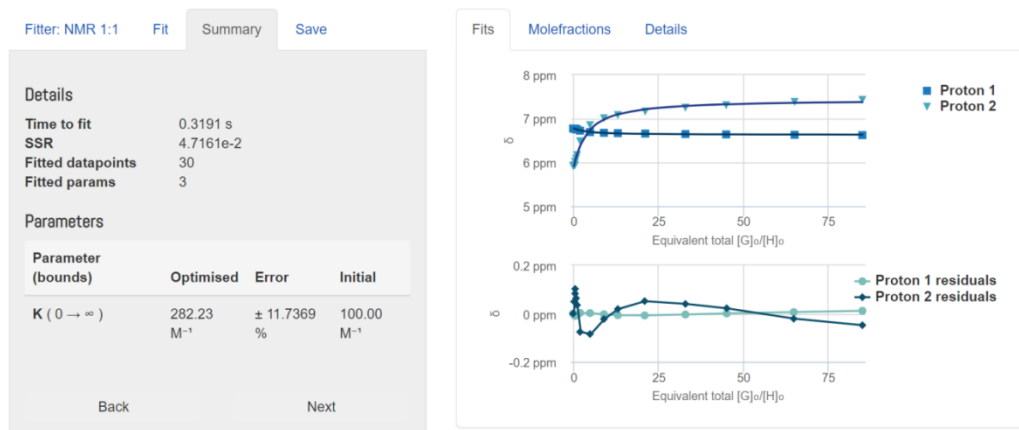
Fig. S56. Nonlinear least-square analysis of the 1 H NMR binding data corresponding to the formation of 1-trans -HP 2 O 7 3- complex. The data extracted from Fig. S55 were fitted to a 1:1 binding model to give K_D = (2.82 \pm 0.33) \times 10^2 \text{ M}^{-1} . The residual distribution is shown below the binding isotherm. All solid lines were obtained from non-linear curve-fitting to a 1:1 binding model using the www.supramolecular.org web applet. 6-8
