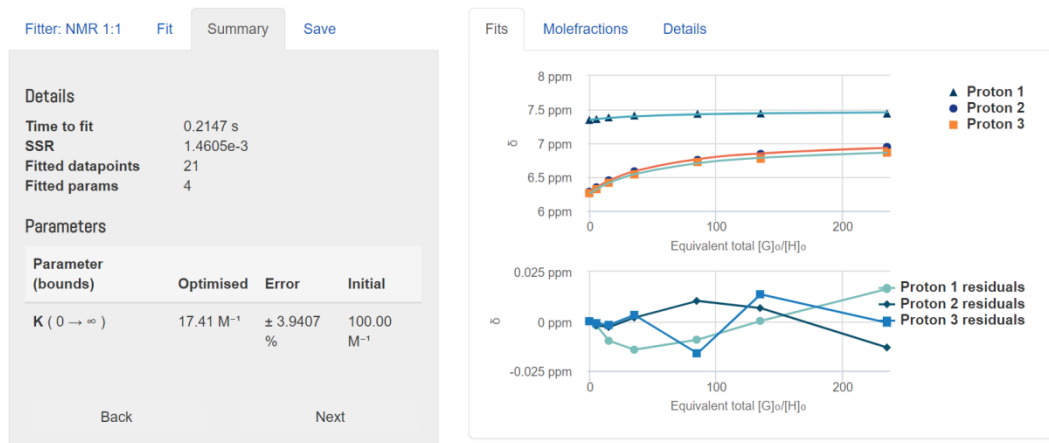
Fig. S38. Nonlinear least-square analysis of the 1 H NMR binding data corresponding to the formation of 1-cis -Cl - complex. The data extracted from Fig. S36 were fitted to a 1:1 binding model to give K_a = (1.74 \pm 0.07) \times 10^4 \text{ M}^{-1} . The residual distribution is shown below the binding isotherm. All solid lines were obtained from non-linear curve-fitting to a 1:1 binding model using the www.supramolecular.org web applet. 6-8
