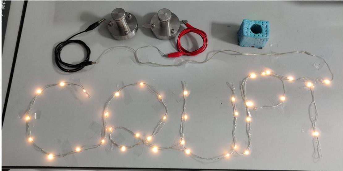
**Fig. S15** Image of  $\text{Fe}_2\text{O}_3\text{-S/ACC/NiCo-PBA}$  ASC device that lighted a series of LEDs
