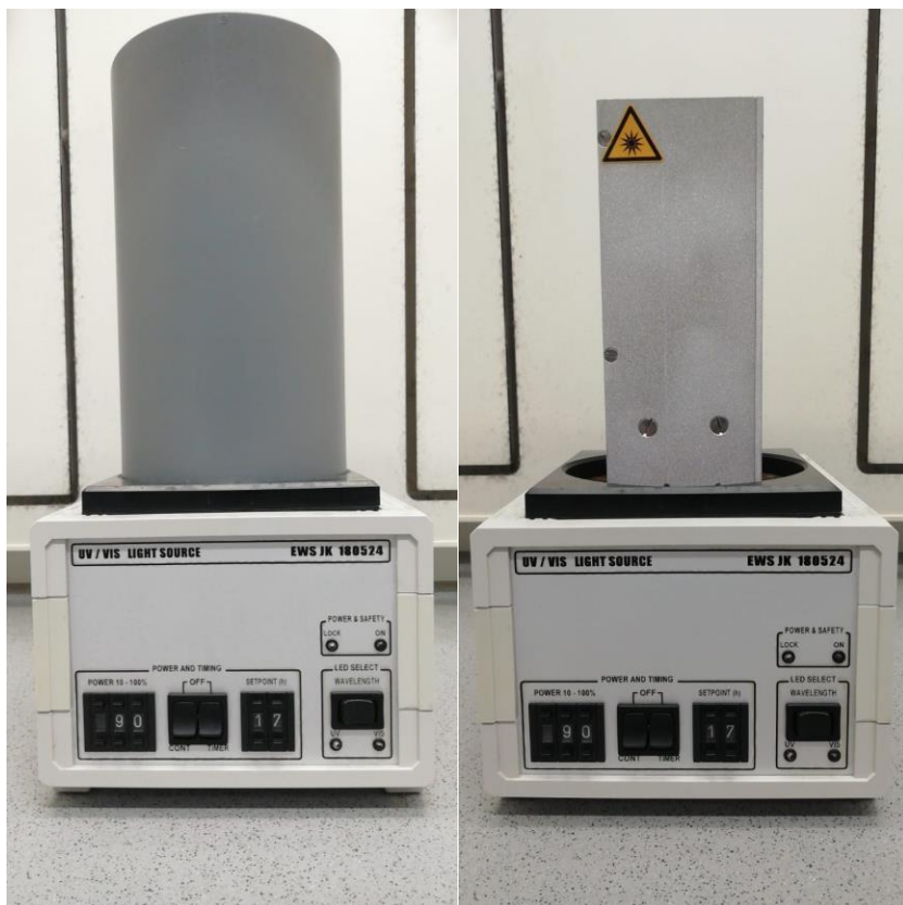
Figure S74: Frontal view (picture) of the UV/vis light source. Closed irradiation chamber (left), open chamber (right).
