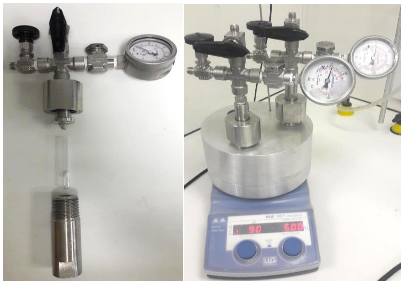
Figure S1 – Small-scale autoclave, disassembled (left), and inside the heating block (right).
