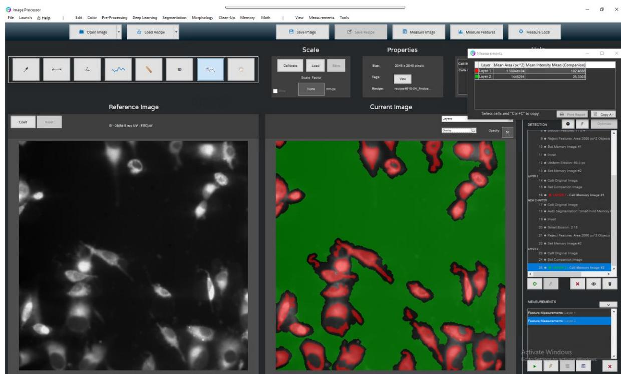
**Figure S13.** Example image of fluorescence quantitation using MIPAR Image Analysis software suite. Results used in **Fig. 2**, **Fig. S12**, **Fig. S13** and **Fig. S14** are the average of 24 fields per condition (6 fields per well in quadruplicate biological replicate), at 7 different concentrations. Cells are shown in red, and background shown in green.
