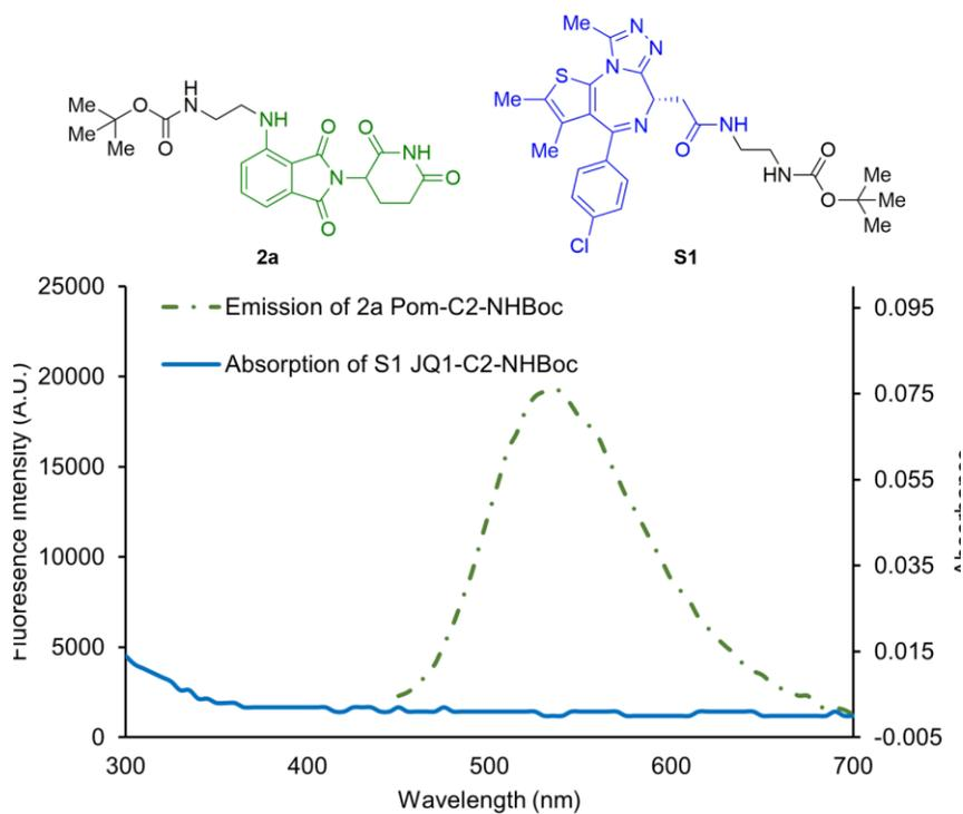
**Figure S9.** Comparison of spectral overlap of JQ1-linker **S1** absorbance and pomalidomide-linker **2a** emission at 415 nm excitation. Spectra were recorded at 10  $\mu\text{M}$  concentration in PBS solution with 2% DMSO.
