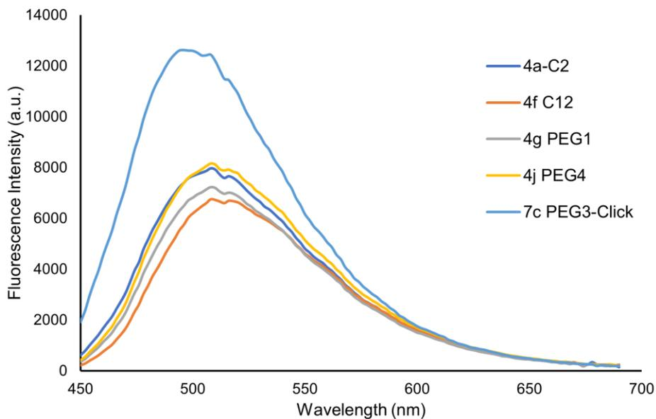
**Figure S7.** Emission spectra of PROTAC library with excitation at 420 nm at 100  $\mu\text{M}$  concentration in ethanol.
