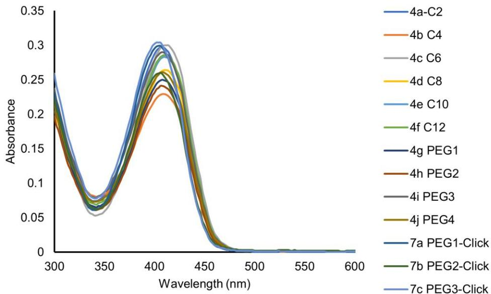
**Figure S2.** UV-visible light absorption of PROTAC library at 100  $\mu$ M concentration in octanol.
