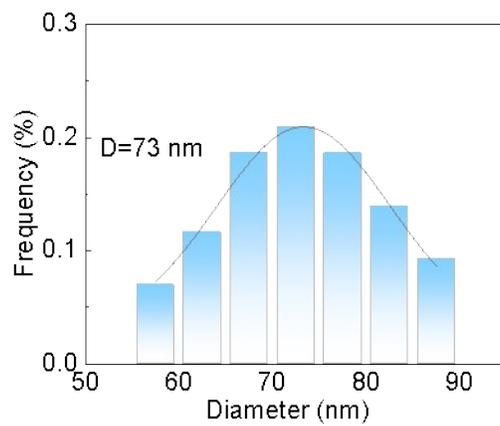
**Fig. S3** Statistical distribution of diameter from optical image of AgNPs.
