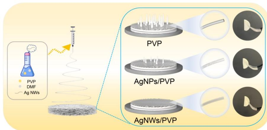
**Fig. S1** Schematic illustration of the synthetic procedure for the PVP, AgNPs/PVP and AgNWs/PVP nanofibers.
