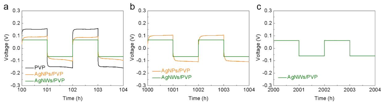
**Fig. S10** Enlarged voltage profiles of the Li||Li symmetric cells with different modified interlayers at 1 mA cm<sup>-2</sup> for 1 mAh cm<sup>-2</sup> after (a) 100 h, (b) 1000 h and (c) 2000 h.
