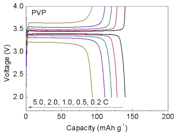
**Fig. S12** The charge/discharge curves at different current densities of the Li||PVP||LFP full cell.
