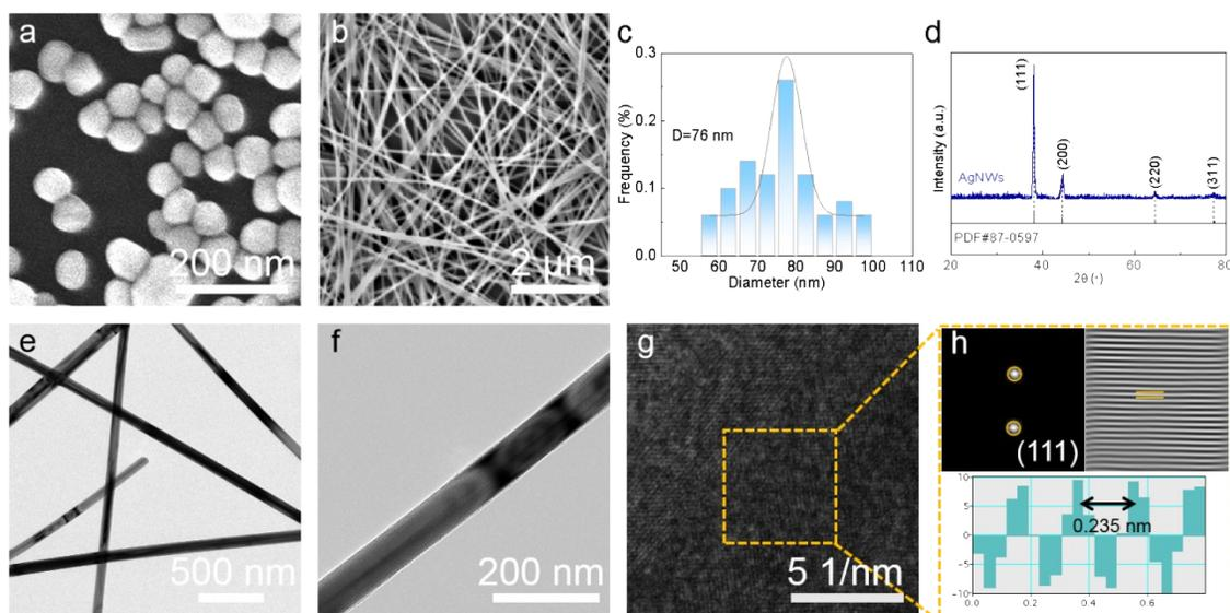
**Fig. S2** SEM images of (a) AgNPs and (b) AgNWs; (c) statistical distribution of diameter from optical image of AgNWs; (d) XRD pattern of AgNWs; (e, f) TEM images in different magnifications, (g) HRTEM image, (h) FFT pattern, IFFT pattern and lattice spacing profile at selected area for AgNWs.
