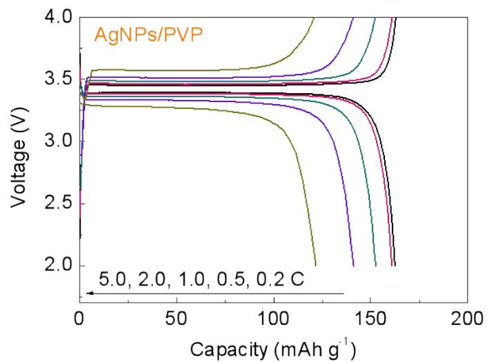
**Fig. S13** The charge/discharge curves at different current densities of the Li||AgNPs/PVP||LFP full cell.
