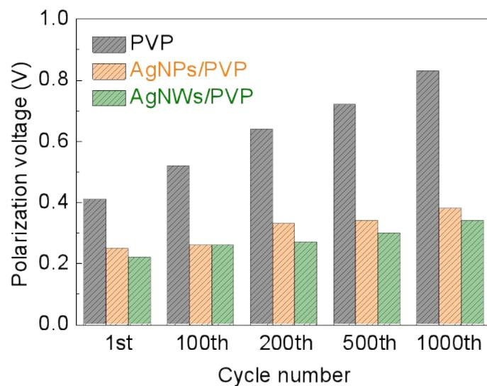
**Fig. S14** Polarization voltage at different cycles of the Li||LFP full cells with PVP, AgNPs/PVP and AgNWs/PVP modified interlayers.
