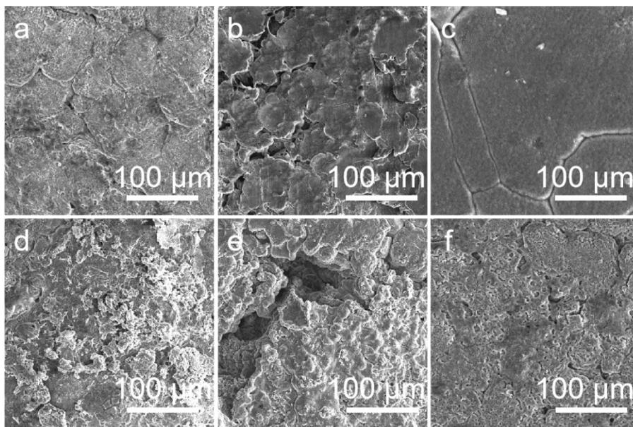
**Fig. S9** SEM images of Li surfaces with (a) PVP, (b) AgNPs/PVP and (c) AgNWs/PVP interlayers after 50 cycles; the SEM images of Li surfaces with (d) PVP, (e) AgNPs/PVP and (f) AgNWs/PVP interlayers after 150 cycles.
