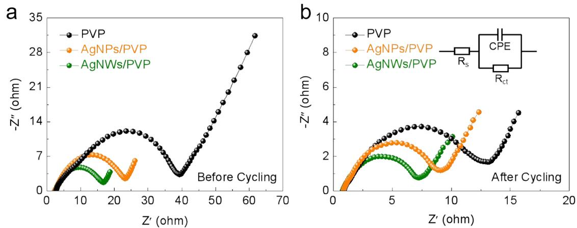
**Fig. S11** EIS plots of Li||Li symmetric cells with different modified interlayers (a) before cycling and (b) after cycling (the inset shows the obtained equivalent circuit).
