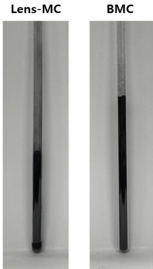
**Figure S13.** The comparison of tap densities of Lens-MC and BMC. 200 mg of each sample was filled in glass tubes with diameter of 5 mm.
