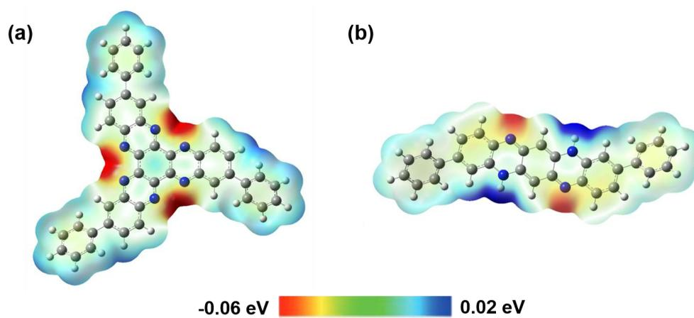
**Fig S19** DFT-optimized ESP profiles of (a) P3Q and (b) TDB.
