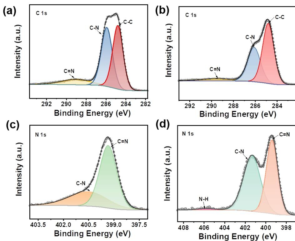
**Fig S5** High-resolution XPS spectra of (a) C 1s and (c) N 1s for P3Q and (b) C 1s and (d) N 1s for TDB.
