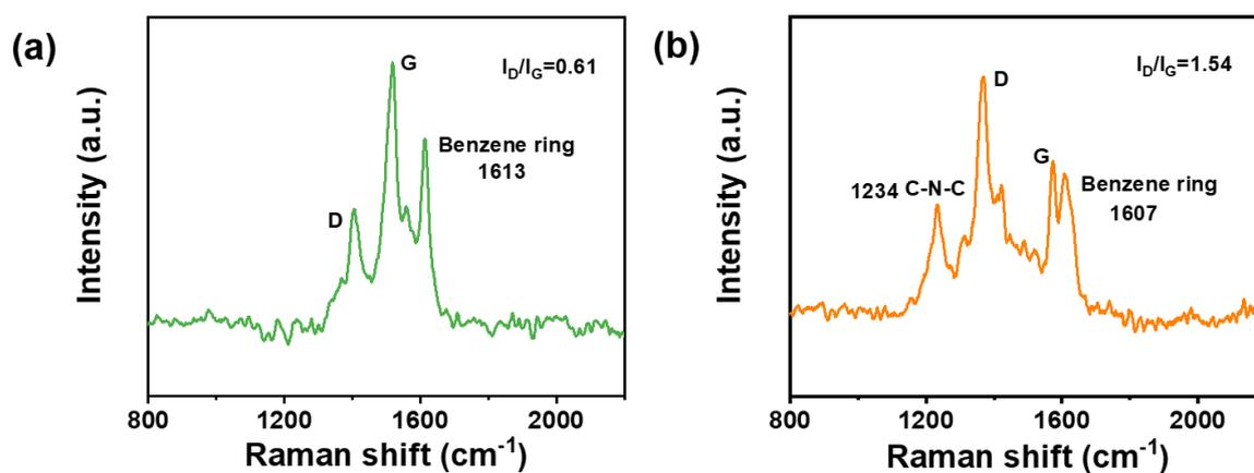
**Fig S7** Raman spectra of (a) P3Q and (b) TDB.
