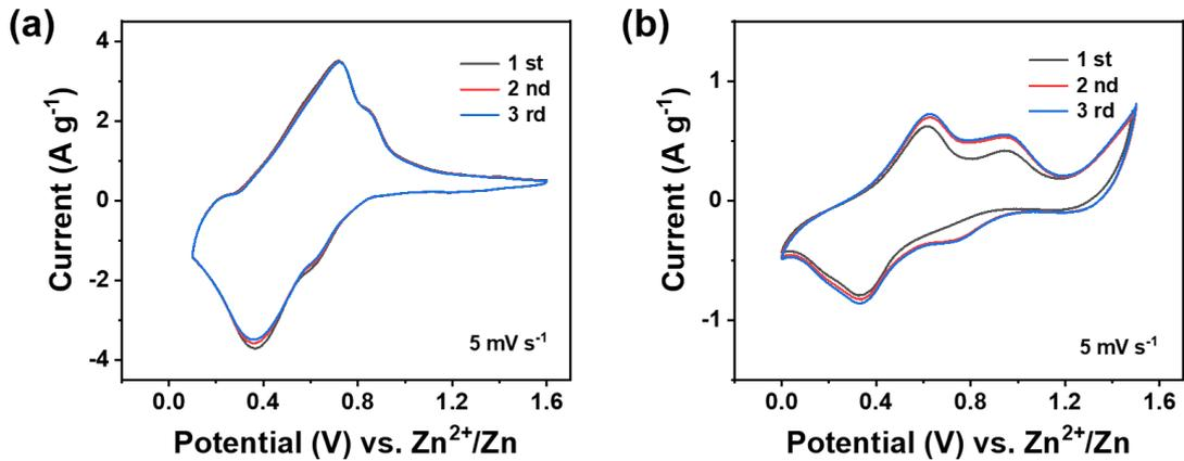
Fig S9 The first three CV curves of (a) P3Q and (b) TDB at 5 mV s<sup>-1</sup>
