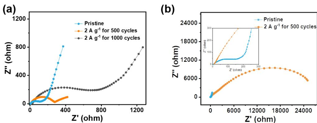
**Fig S14** Impedance spectra of (a) P3Q and (b) TDB before and after GCD cycles.
