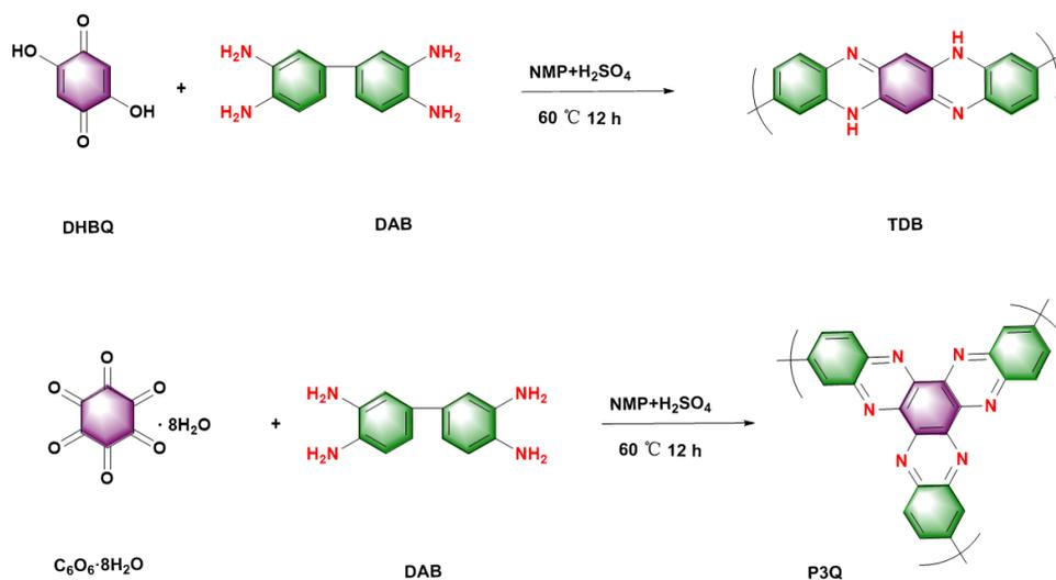
Fig S1 The synthetic procedures of TDB and P3Q.
