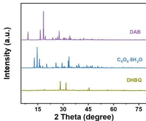
**Fig S4** XRD curves of DAB,  $C_6O_6 \cdot 8H_2O$  and DHBQ.
