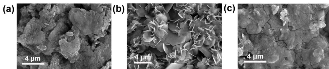
**Fig S16** The *ex situ* SEM images of P3Q electrodes at (a) pristine, (b) discharged and (c) charged states at  $0.1 \text{ A g}^{-1}$ .
