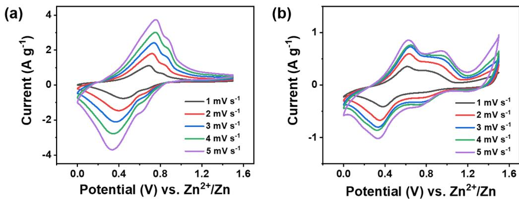
Fig S11 CV curves of (a) P3Q and (b) TDB at various sweep rates in ZIBs.
