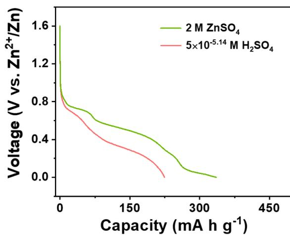
**Fig S18** GCD curves at  $0.1 \text{ A g}^{-1}$  of P3Q in two kinds of electrolytes.
