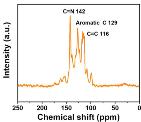
Fig S3 Solid-state  $^{13}\text{C}$  NMR spectra of TDB.
