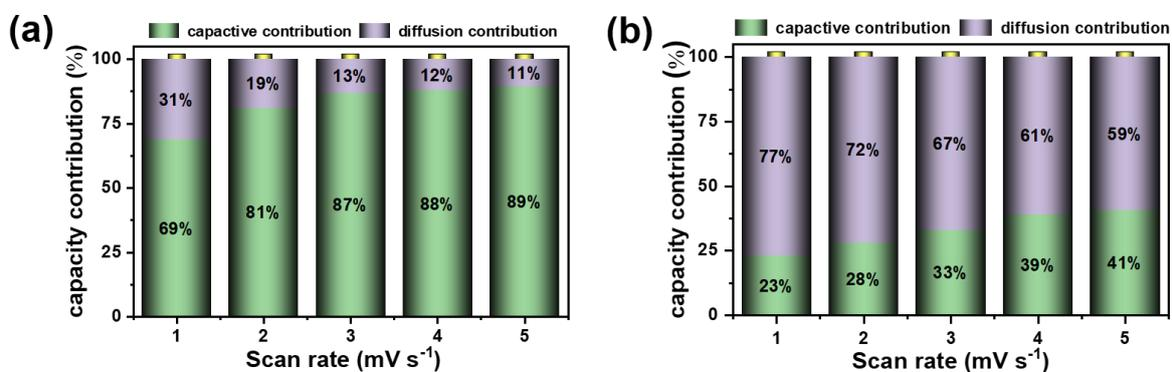
**Fig S13** The ratio of capacitance control and diffusion control for (a) P3Q and (b) TDB at different scan rates.
