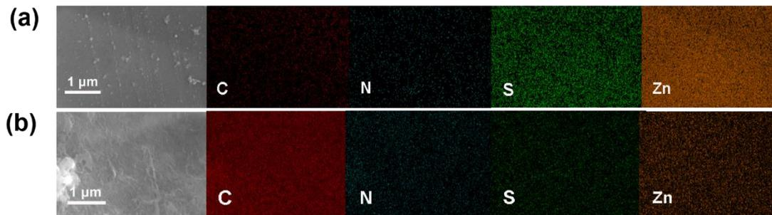
**Fig S15** SEM-EDS mapping of C, N, S, and Zn elemental distributions of P3Q electrodes at (a) discharged and (b) charged states at  $0.1 \text{ A g}^{-1}$ .
