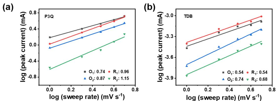
**Fig S12** Determination of  $b$  value from the logarithm of oxidation/reduction peak current versus logarithm of scan rate for (a) P3Q and (b) TDB.
