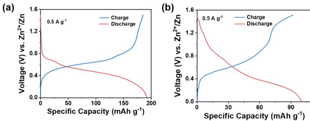
Fig S10 The charge/discharge curves of (a) P3Q and (b) TDB at 0.5 A g<sup>-1</sup>
