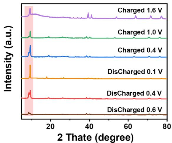
**Fig S17** The XRD pattern of P3Q cathode in ZIBs at different GCD states.
