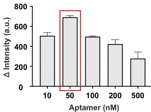
**Fig. S8.** Effect of aptamer concentration on signal response. When the aptamer concentration was 50 nM, the signal change was maximum. The PSA concentration was constantly 10 ng/mL. Error bars, mean  $\pm$  s.d. (n = 3).
