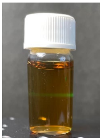
Fig. S3 Photograph of the colloidal dispersion of Co-n.s. A green laser was used to show the Tyndall effect.
