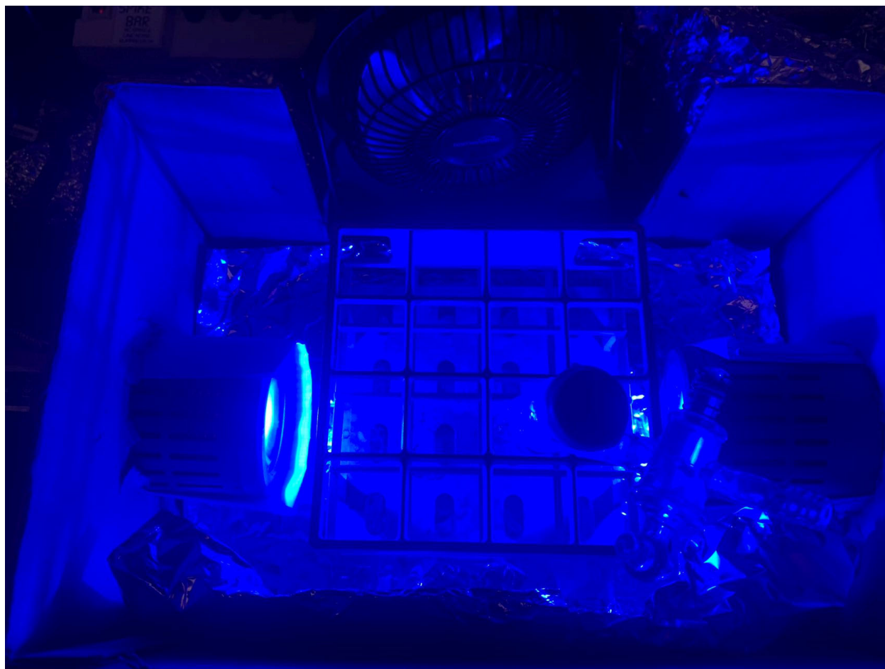
Figure S1. The Visible-Light Photoredox Catalysis Experimental Setup
