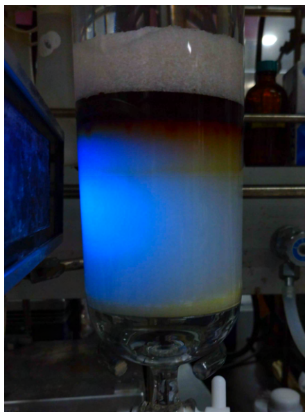
Fig. S1. Picture of silica gel column chromatography irradiated with a 365 nm UV lamp. Fraction with light blue fluorescence contains compound 1 .
