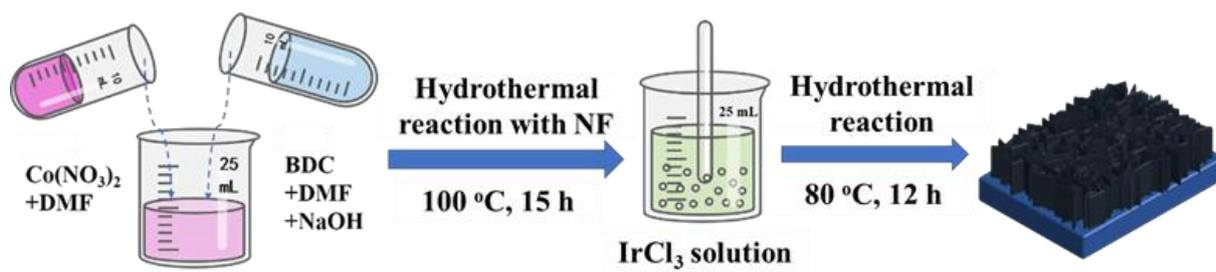
**Figure S1.** Schematic illustration of the synthetic process of CoIr<sub>x</sub>-BDC.
