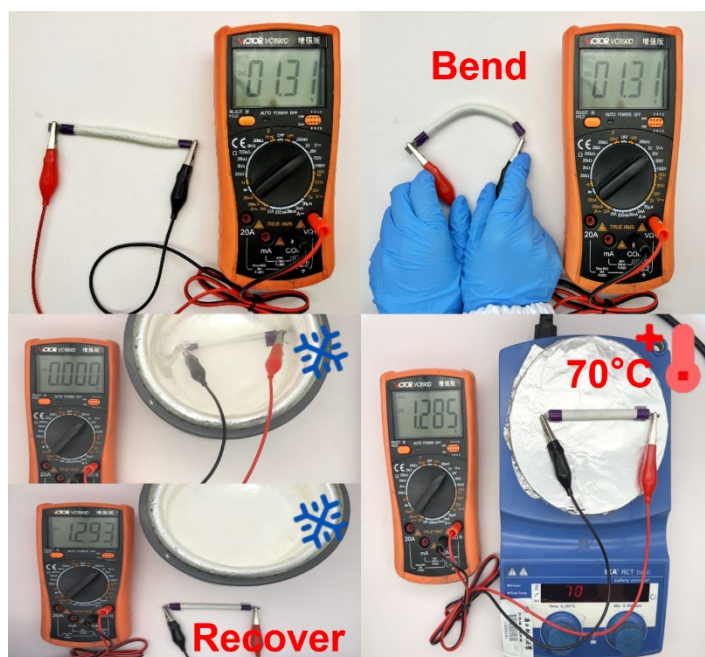
Fig. S16 OCV plots of FZABs in various conditions: room temperature, bending, freezing in liquid nitrogen, and heating.
