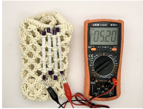
Fig. S17 The OCV of four FZABs knitted in a woven bag.
