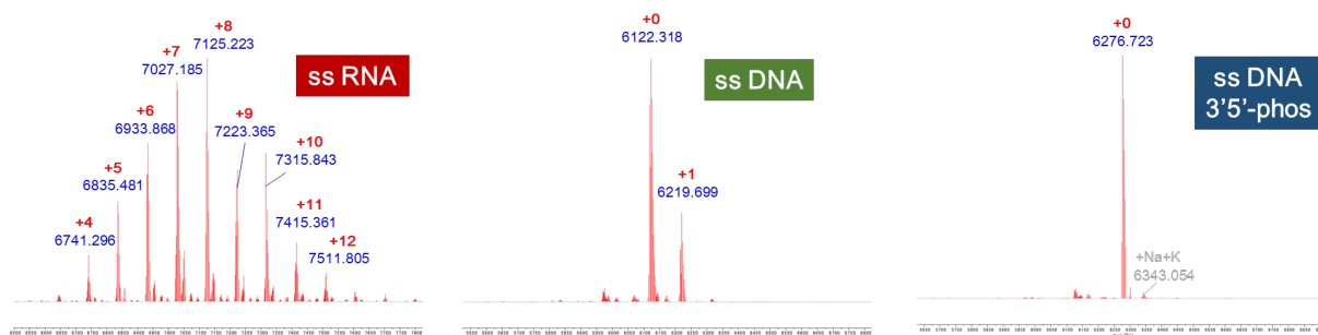
Figure S7. Comparison of acylation reactivity of ssRNA (left) and ssDNA (center and right) with cyclobutanone acylating reagent 14 . The tests show that 14 is OH group selective, and does not react with exocyclic groups on bases. The small amount of reactivity for DNA (center) is absent when the 5' and 3' OH groups on the ends are blocked (right). Conditions: RNA (DNA) 10 \mu M, acylimidazole 200 mM, MOPS buffer pH 7.5, 0°C, 2 h.
