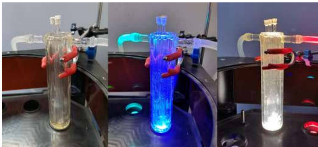
Figure S21. Experimental setup for irradiation of NMR tubes.
