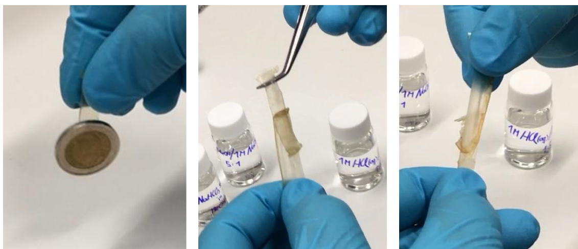
Figure S8. Pictures demonstrating the adhesion of the A- and C-grafted polymer surfaces. Left: lifting a 2 euro coin after contact with the treated surface. Middle and right: contact of A- and C-grafted polymer surfaces followed by stretching.
