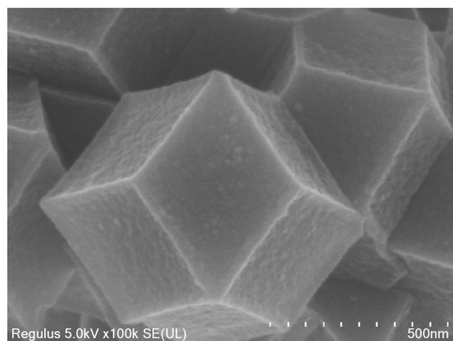
**Figure S2.** The SEM image of ZIF-C with high magnification.
