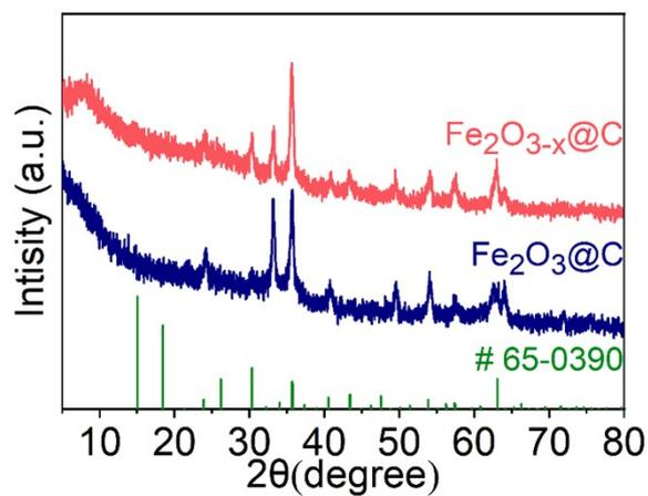
**Figure S5.** The XRD results of the  $\text{Fe}_2\text{O}_3@\text{C}$  and  $\text{Fe}_2\text{O}_{3-x}@\text{C}$ .
