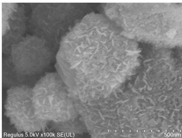
**Figure S3.** The SEM image of FeOOH@C.
