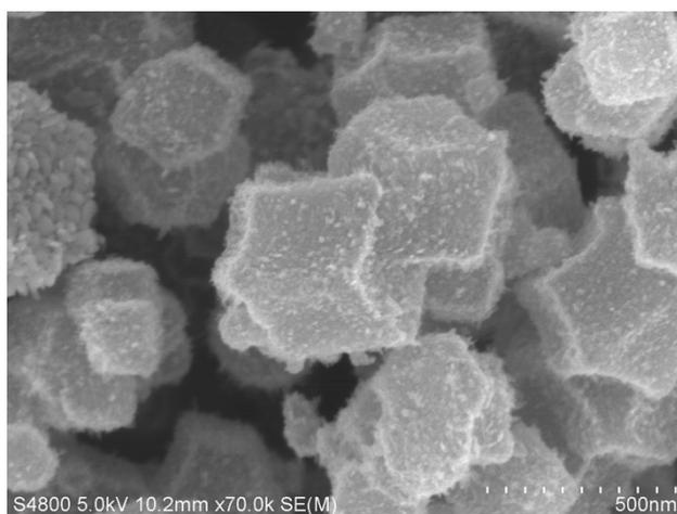
**Figure S4.** The SEM image of Fe<sub>2</sub>O<sub>3</sub>@C.
