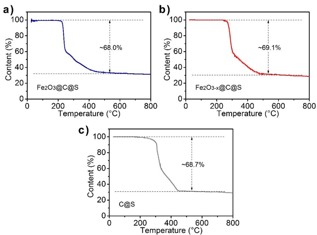
**Figure S6.** TGA results of (a)  $\text{Fe}_2\text{O}_3@\text{C}@\text{S}$ , (b)  $\text{Fe}_2\text{O}_{3-x}@\text{C}@\text{S}$  and (c)  $\text{C}@\text{S}$ .
