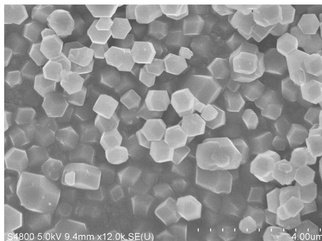
**Figure S1.** The SEM image of ZIF-8.
