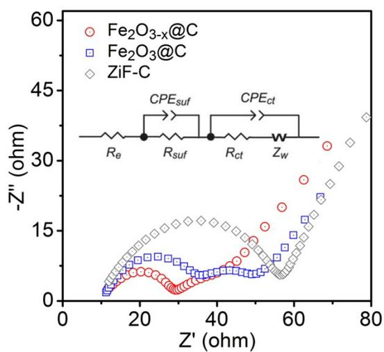
**Figure S7.** EIS results and corresponding fitted equivalent circuit model of  $\text{Fe}_2\text{O}_{3-x}@C@S$ ,  $\text{Fe}_2\text{O}_3@C@S$ , and ZiF-C@S cathodes.
