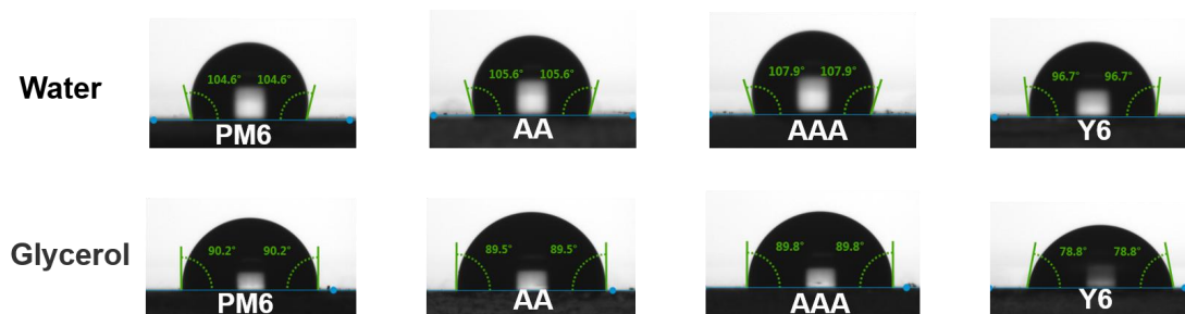
Figure S9. Contact angles of drops of water and glycerol for surface energy analysis of PM6, AA, AAA, Y6
