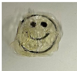
Figure S1. Film made by drop casting the viscous solution of 10 on a Teflon mold.
