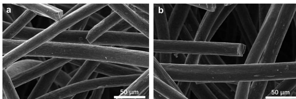
**Figure S8** SEM images of the GF cathode (a) before the experiment; (b) after 5 cycles of the electrochemical reaction.
