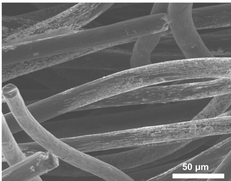
**Figure S7** SEM images of the prepared  $\text{CoS}_2/\text{CoS}@\text{GF}$  heterojunction electrode after 5 cycles of the electrochemical reaction.
