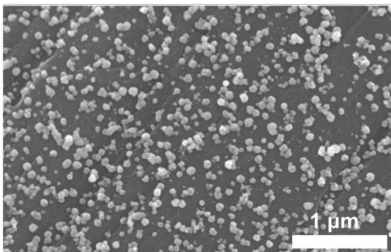
**Figure S5 (a)** High-resolution SEM image of  $\text{CoS}_2/\text{CoS}@GF$  electrode.
