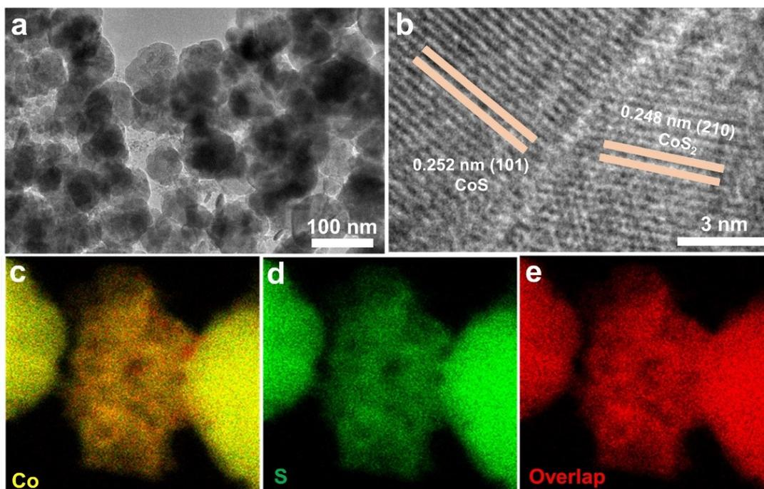
Figure S2 (a) TEM image and (b) High-resolution TEM image of  $\text{CoS}_2/\text{CoS}$  heterojunction, (c-e) elemental mappings of Co and S.
