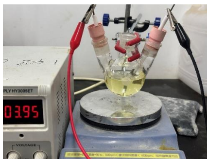
Figure S2 Gram-scale amplification Electrolysis setup
