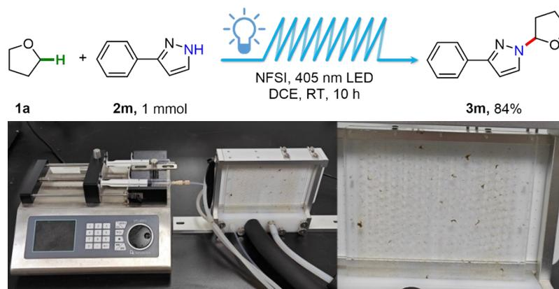
Figure S5. Continuous-Flow Reaction Setup
