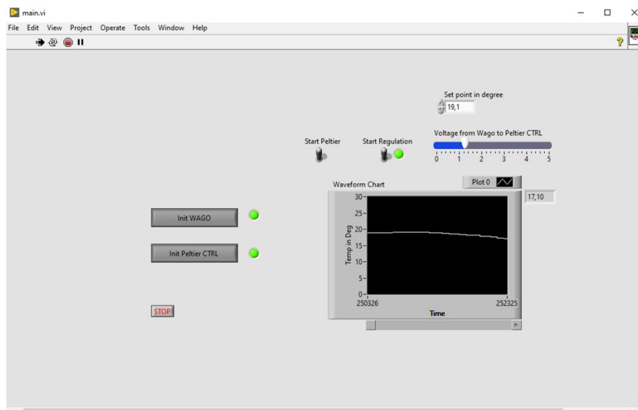
Figure S6 The GUI of the LabVIEW software developed for thermal regulation of the microchips. The interface includes buttons to initialize the controller and the WAGO system, to set the temperature (°C) and start the regulation of the Peltier module.
