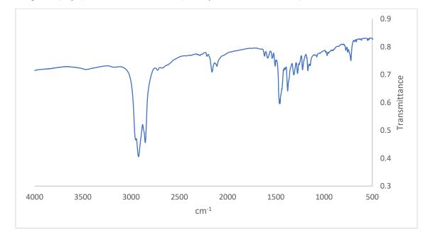
FT-IR spectra (Nujol) of TAPP in its 2T form (the only tautomer in solid state)
