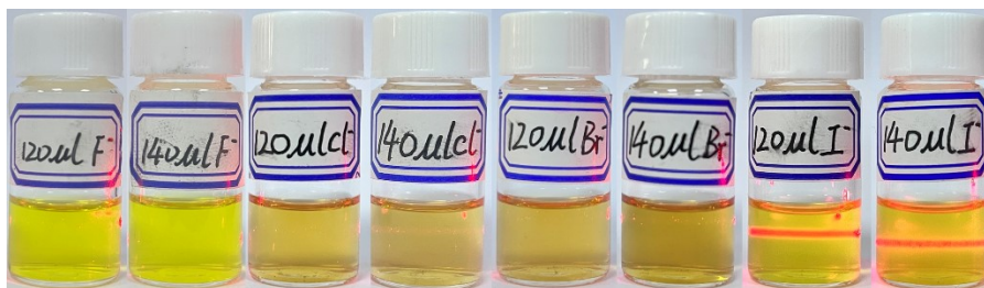
Figure S4. Pictures of solutions of \{Ag_{32}S_3\} with different halogen ions added under laser pointer illumination.
