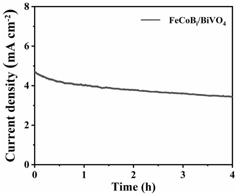
Fig. S6. The stability test curves of CoFeBi/BiVO<sub>4</sub> electrodes.
