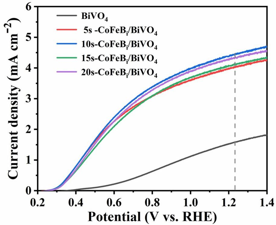
Fig. S2. LSV curves of CoFeB<sub>7</sub>/BiVO<sub>4</sub> with different deposition time.
