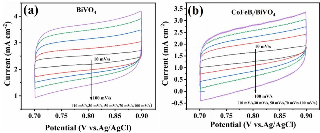
Fig. S3. CV of photoanodes performed at different scan rates in the non-Faradaic potential range.
