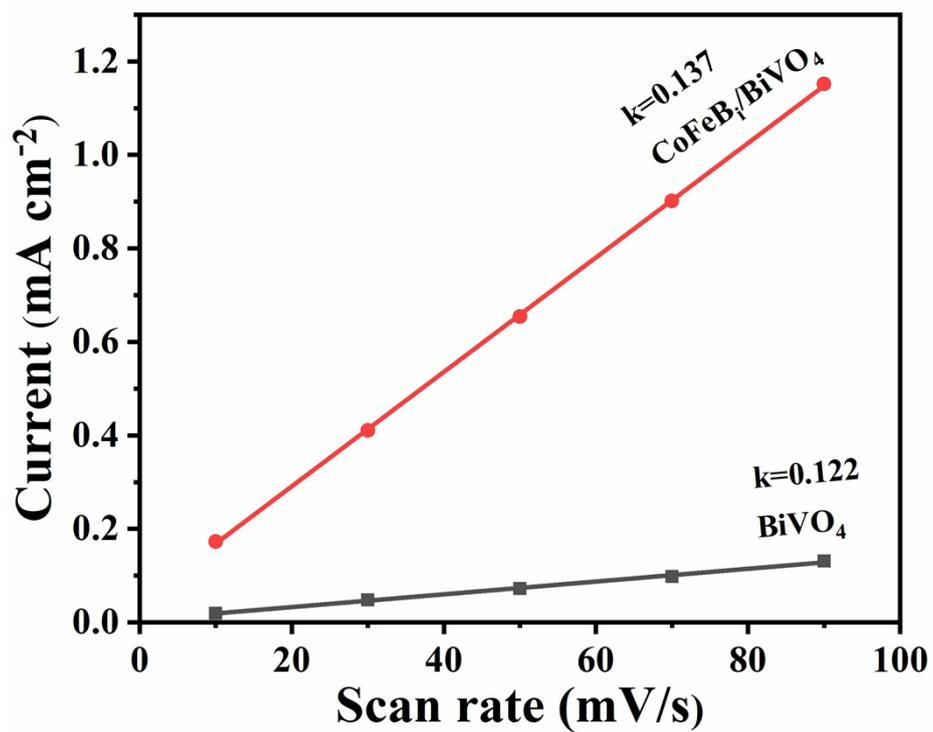
Fig. S4. Relationship between current density difference and scan rate of BiVO<sub>4</sub> and CoFeBi/BiVO<sub>4</sub> photoanodes.
