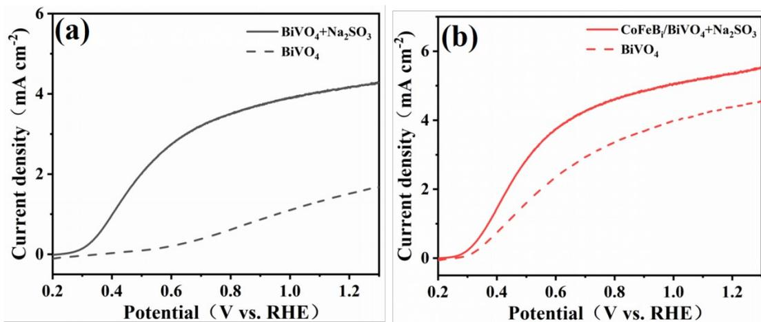
Fig. S5. BiVO<sub>4</sub> and CoFeBi/BiVO<sub>4</sub> electrodes measured by in 1 M Na<sub>2</sub>SO<sub>3</sub> solution of linear sweep voltammetric curves (a), (b).
