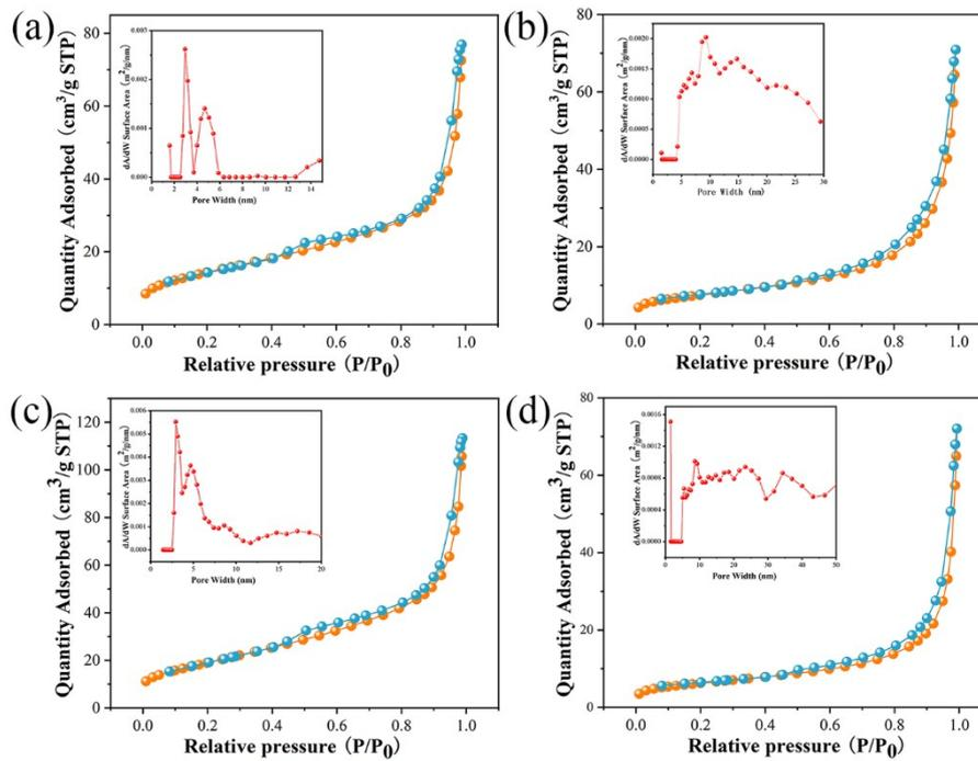
Fig. S3.  $N_2$  adsorption/desorption isotherms and pore-size (inset) distributions of (a) CoNi-1, (b) CoNi-F, (c) CoNi-rGO, (d) S-CoNi-rGO, respectively.
