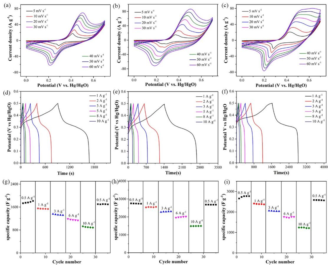
Fig. S4. (a-c) CV curves at different scan rates, (d-f) GCD curves at different current densities, (g-i) the cycling performance at various current densities of CoNi-1, CoNi-F, CoNi-rGO.
