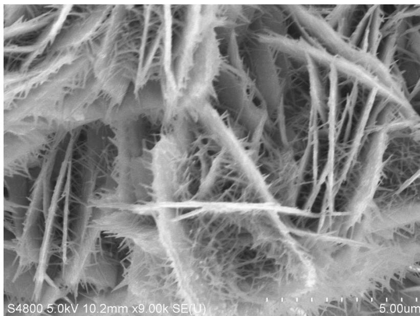
Fig. S7. The SEM images of S-CoNi-rGO // AC ASC device after 5000 cycles tests.
