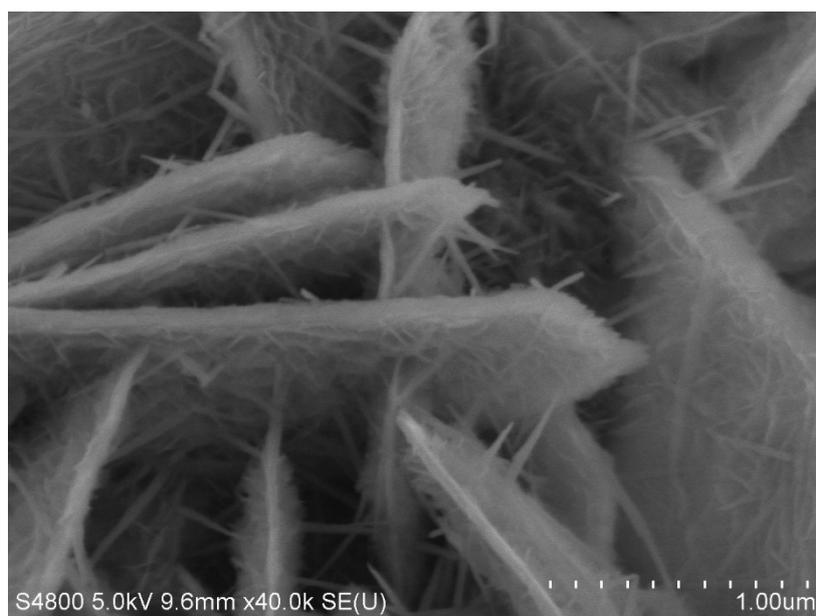
Fig. S6. The SEM images of S-CoNi-rGO after 10000 cycles tests.
