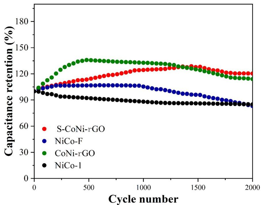
Fig. S5. The cycling stability for CoNi-1, CoNi-F, CoNi-rGO and S-CoNi-rGO at current density of 10 A g<sup>-1</sup>.
