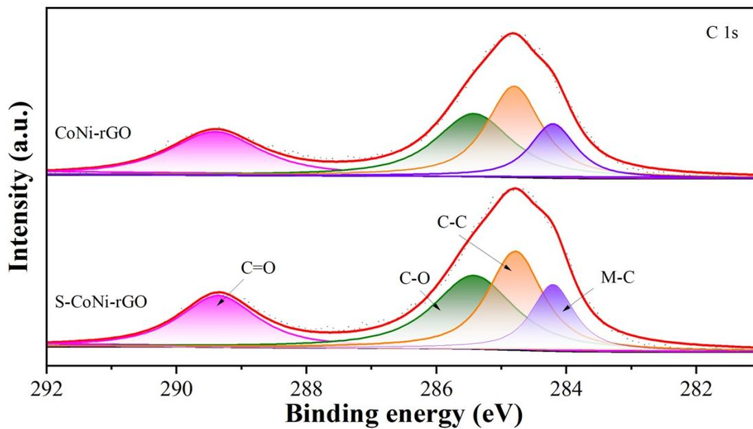
Fig. S1. XPS spectra of CoNi-rGO, S-CoNi-rGO for C 1s.
