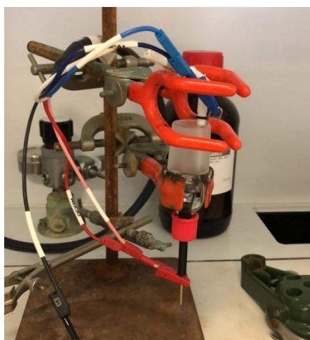
Figure S20. Solid state cyclic voltammetry set-up (left: set-up picture, right: schematic representation).
