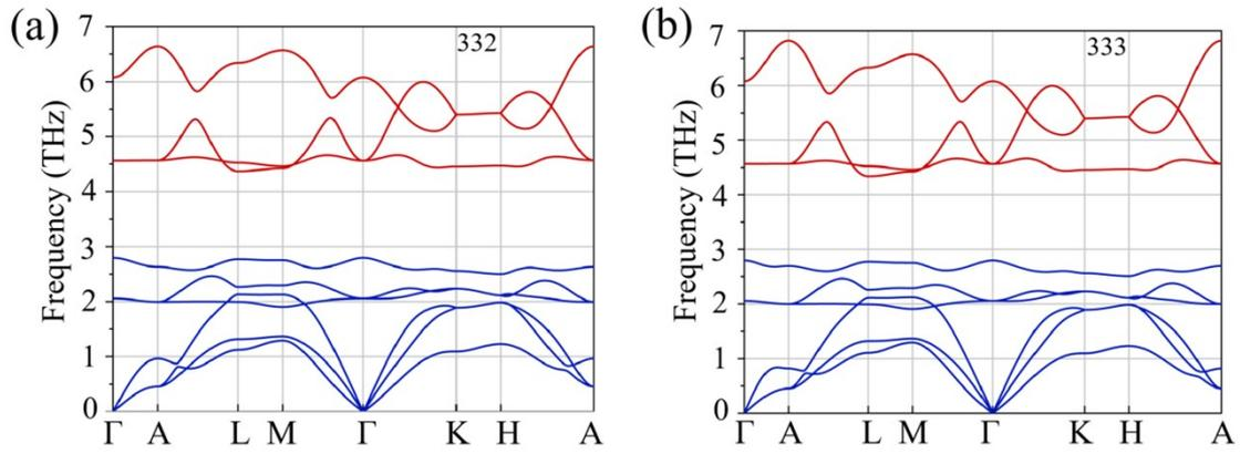
Figure S2. Phonon spectra of  $\text{CaI}_2$  for the  $3 \times 3 \times 2$  supercell (a) and the  $3 \times 3 \times 3$  supercell (b).
