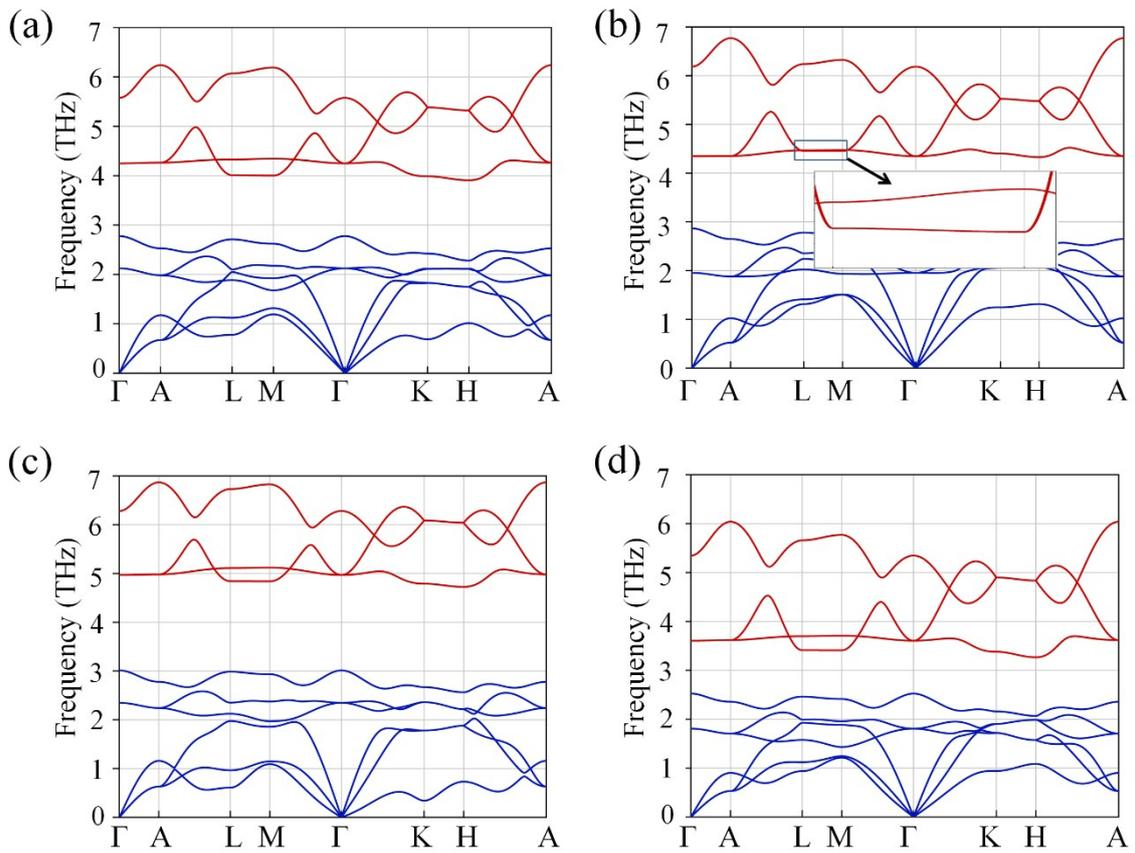
Figure S3. The computed phonon spectra of  $\text{CaI}_2$  under -3% uniaxial strain on the  $c$  axis (a), +3% uniaxial strain on the  $c$  axis (b), -2% uniform strain (c) and +2% uniform strain (d). The inset in (b) is an enlarge view for the rectangle.
