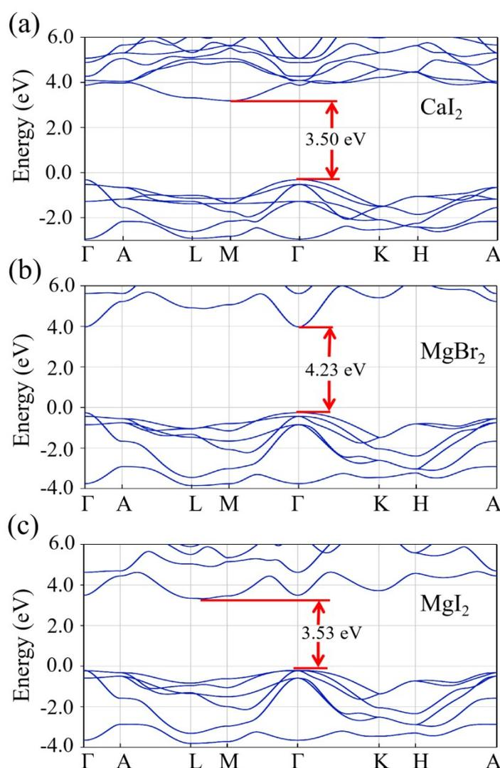
Figure S1. Band structures of  $\text{CaI}_2$  (a),  $\text{MgBr}_2$  (b) and  $\text{MgI}_2$  (c). One can find  $\text{CaI}_2$ ,  $\text{MgBr}_2$  and  $\text{MgI}_2$  are semiconductors with an indirect gap 3.50 eV, a direct gap 4.23 eV and an indirect gap 3.53 eV, respectively.
