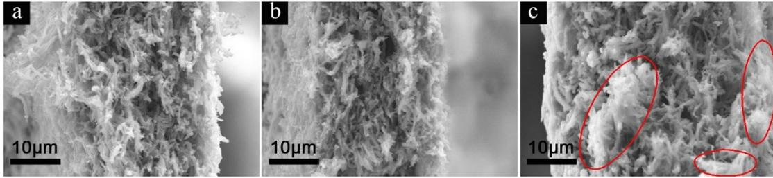
Figure S9 Cross-section of flexible porous PPy films after cycle measurement, PPy film@N1.5/E1.5 (a), PPy film@N1.5/E3 (b), PPy film@N1.5/E6 (c)
