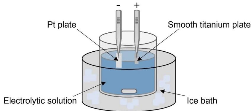
Figure S5 Schematic for preparation of compact PPy film
