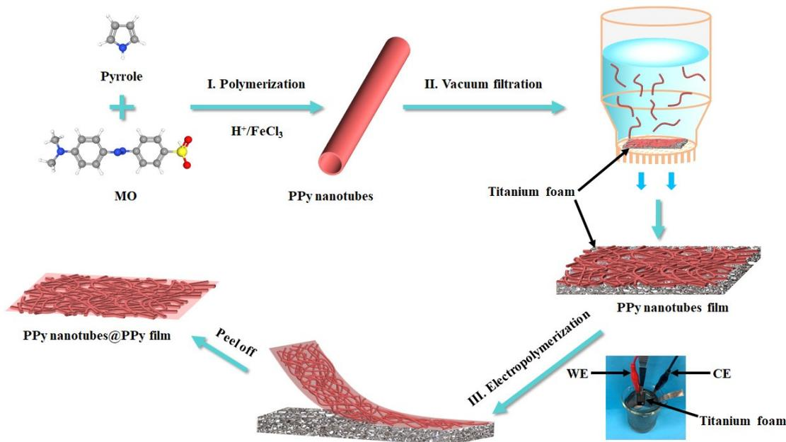
Figure S3 Schematic for preparation of flexible porous PPy film
