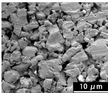
Figure S4 Morphology of porous titanium plate
