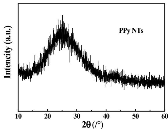
Figure S2 X-ray diffraction patterns of PPy NTs
