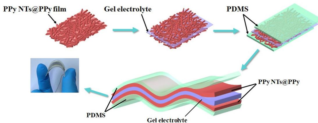
Figure S6 Schematic for fabrication of flexible supercapacitors
