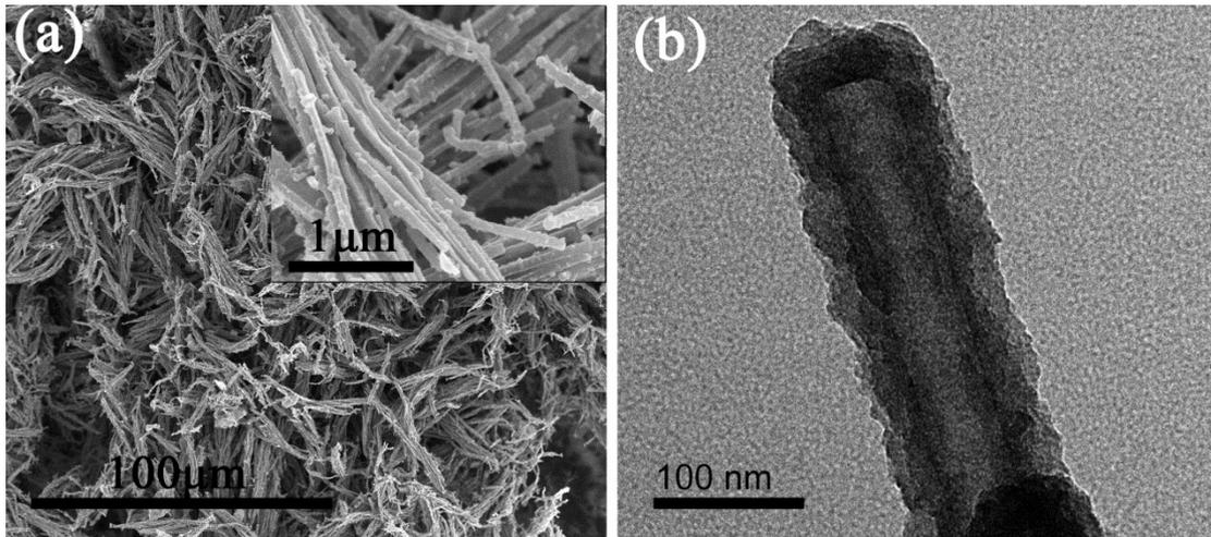
Figure S1 Morphology and microstructure of PPy NTs
