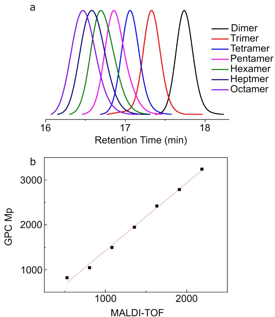
**Figure S5.** (a) GPC traces of the final oligomers with tabulated number and weight average mass versus polystyrene standards. (b) Oligomers obtained by GPC plot against mass values obtained by MALDI-TOF, a straight line of best fit (red) revealed a gradient and therefore a conversion factor of 1.51 between the two techniques.
