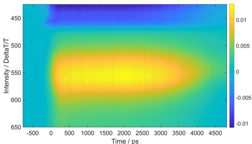
**Figure S4: Transient absorption spectroscopy of the  $n = 3$  nTV.** Full false colour map of  $n = 3$  nTV after 475 nm excitation in (OD  $\sim 0.3$ , 1 mm path length) toluene solution.
