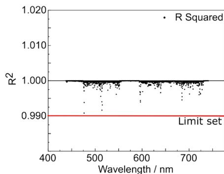
**Figure S3: R value associated with the global fitting at each wavelength.** Result of the global analysis was considered unsuccessful unless all fits have an  $R^2$  value of 0.99 or more (labelled as a red line).
