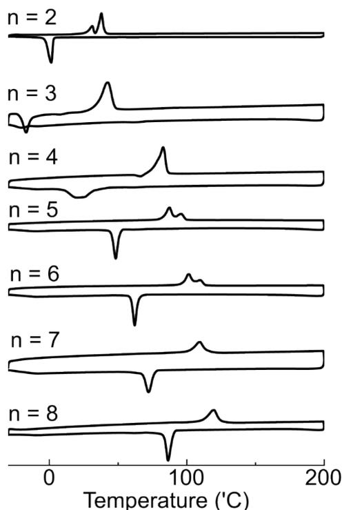
**Figure S15.** DSC plots (endotherm up), second cycle (10 °C/min).
