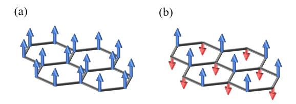
**Fig. S1** (Color online) (a) The ferromagnetic configuration of VS<sub>2</sub>, where the total energy can be written as:  $E_1 = E_0 - \frac{1}{2} \cdot \frac{1}{2} \cdot 3 \cdot 16 \cdot J = E_0 - 6J.$ (b) Antiferromagnetic configuration of VS<sub>2</sub>, where the total energy can be written as:  $E_2 = E_0 + \frac{1}{2} \cdot \frac{1}{2} \cdot 3 \cdot 16 \cdot J = E_0 + 6J$ . Here,  $E_0$  is the total energy excluding the
