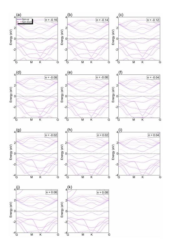
**Fig. S2** (Color online) (a)-(g) Band structure at different hole concentrations; (h)-(k) Band structure at different electron concentrations. The purple lines represent spin-up bands and the red lines represent spin-down bands.
