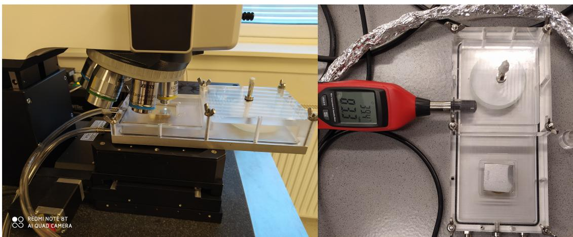
Figure S1: Home-made cell for In-situ Raman analysis. Schematic representation (top), set-up used during in-situ measurements and top view of the cell used for in-situ measurements (bottom). In the bottom right picture it is also shown the temperature and humidity sensor. Approximate dimensions are schematically indicated in the top image. The width of the cell (not shown in the top image) is 10 cm.
