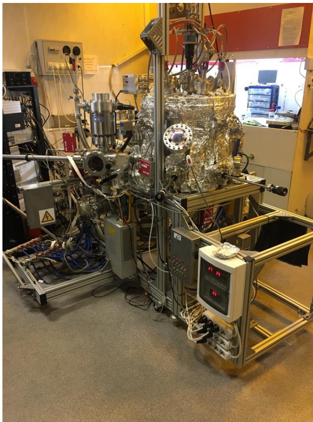
Supplementary Fig. 7. The general view of the ultra-high vacuum sputtering facility utilized in the study.
